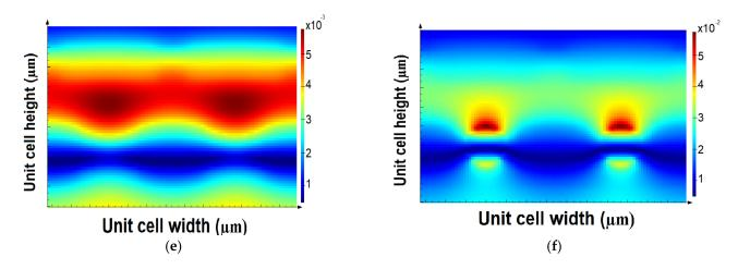
**Figure 10.** Optical power distribution on vertical planes (**a**) for the first monitor, *M*1 (**b**) for the second monitor, *M*2, electric field distribution (**c**) for the first monitor, *M*1 (**d**) for the second monitor, *M*2, and magnetic field distribution (**e**) for the first monitor, *M*1 and (**f**) for the second monitor, *M*2.
