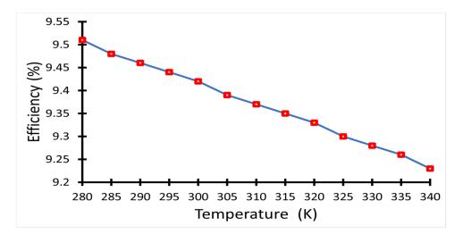
Figure 7. PCE of the solar cell as a function of temperature.
