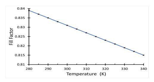
Figure 6. Fill factor of the solar cell as a function of temperature.
