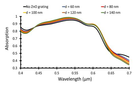
Figure 2. Absorption of different ZnO grating periods versus optical wavelength.
