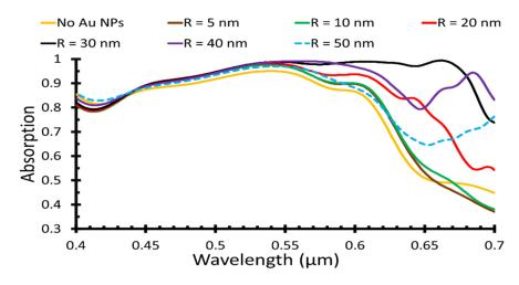
Figure 3. The light absorption of different AuNP radii with the wavelength.
