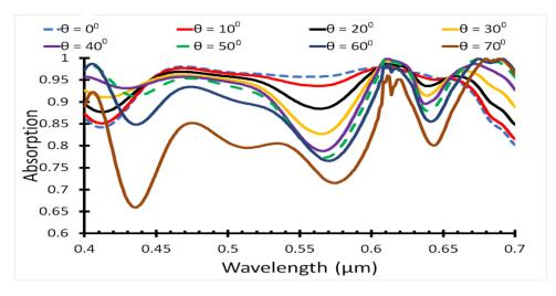
Figure 8. Absorbed light in the active region for different incident angle.
