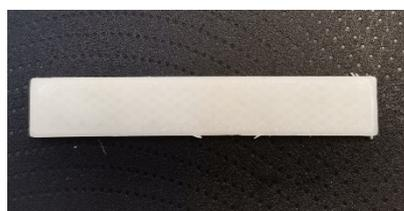
**Figure 1.** Macrograph of FOMM printed test specimen for flexural tests.
