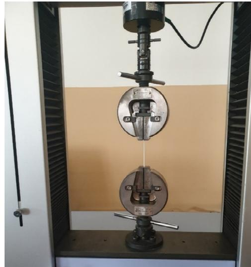
**Figure 2.** Representative macrograph of tensile test of the FOMM filaments.
