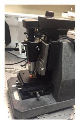
Figure 3. AFM measurements setup.
