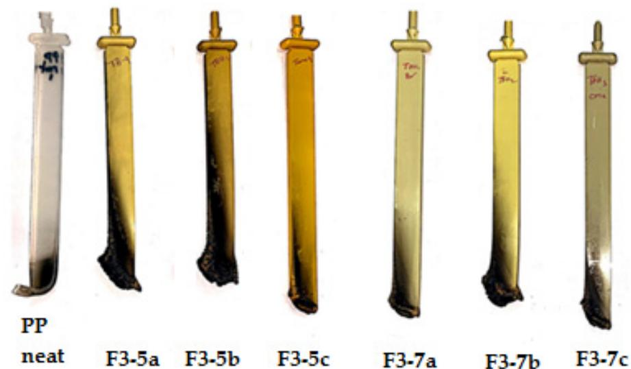
**Figure 10.** Flammability test of PP composites.**Table 6.** Comparison of the flammability characteristics of the prepared polymers with other materials.
