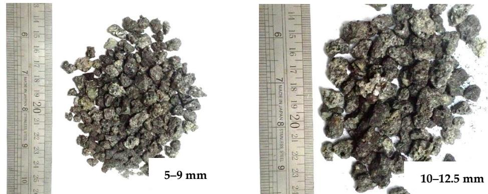
**Figure 2.** Waste POC coarse aggregate.
