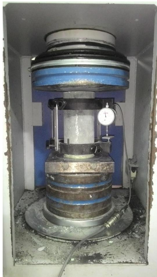
**Figure 5.** Experimental setup for MOE test.
