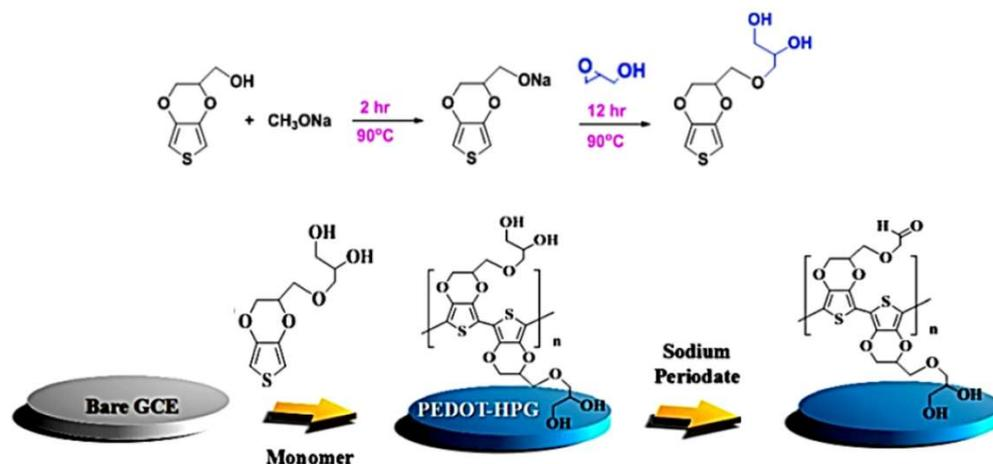
**Scheme 7.** Synthesis of new EDOT-based monomer (top), and electrochemical oxidative polymerization of PEDOT-graft-HPG (bottom). Reproduced with permission from reference [68], copyright (2019), Elsevier.
