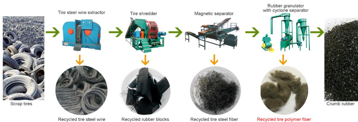
**Figure 4.** The sketch of the scrap tire recycling process.
