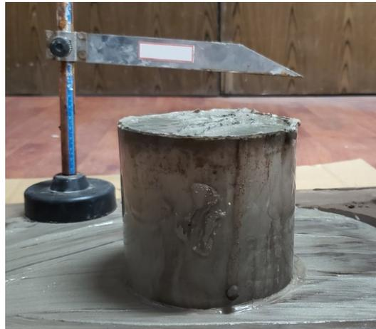
**Figure 7.** Pictorial view of the cylindrical slump test device in this study.
