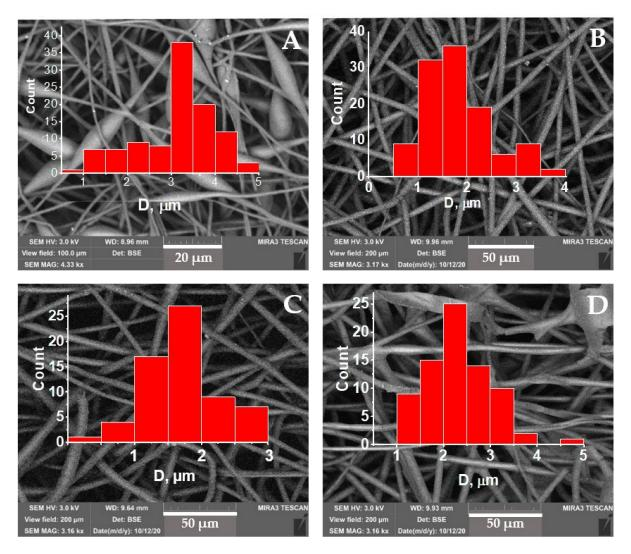
**Figure 2.** SEM images of the PHB fibrillar structures loaded by the metal-porhyrine complex of SnCl<sub>2</sub>. The concentration of SnCl<sub>2</sub>—PPT: (**A**) 0%, (**B**) 1%, (**C**) 3%, (**D**) 5%.
