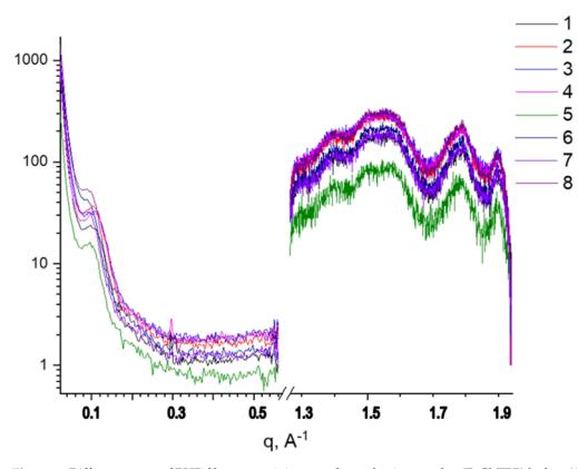
**Figure 3.** Diffractograms of PHB fibers containing metal-porphyrin complex (FeCl-TPP) before (1–4) and after annealing (5–8). PHB: nonannealed (1) and annealed (5); PHB-TPP-FeCl (1%): nonannealed (2) and annealed (6); PHB-TPP-FeCl (3%): nonannealed (3) and annealed (7); PHB-TPP-FeCl (5%): nonannealed (4) and annealed (8).
