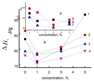
**Figure 9.** Dependence of melting enthalpy on the SnCl<sub>2</sub>-TPP (**a**) and TPP (**b**) content. Durability of water treatment (in min) at 70 °C: 1–0, 2–30, 3–120, 4–240, 5–0, 6–120, 7–240.
