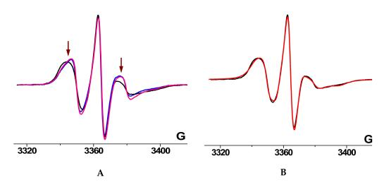
**Figure 5.** EPR spectra changes after annealing at 140 °C. (**A**) EPR spectra of TEMPO radical in PHB samples containing 5% TPP, before annealing (blue line) and after annealing for 90 (pink line) and 240 min (black line). The spectra are normalized to the intensity of the central component; the arrows indicate the regions of the greatest change in the line shape. (**B**) Spectrum simulation for the samples annealed for 240 min (black line—experimental spectrum, red line—simulation result).
