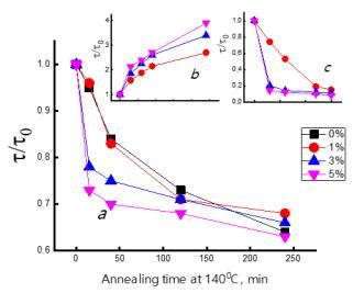
**Figure 7.** Dependence of the molecular dynamics expressed as relative correlation time  $(\tau/\tau_0)$  from annealing time at 140 °C for the PHB electrospun fibers with (a) TPP, (b) SnCl<sub>2</sub>-TPP, (c) FeCl-TPP.
