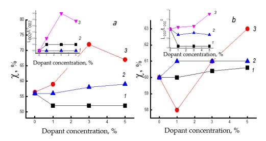
**Figure 4.** Crystallinity degree ( $\chi$ ) dependence and relative longitudinal size ( $L_{00}2/L_{00}^0$ ) evolution (the inserts) as functions of the dopant concentration. (**a**) initial fibers, (**b**) the same fibrous samples after annealing at 140 °C. 1—TPP, 2—SnCl<sub>2</sub>-TPP, 3—FeCl-TPP.
