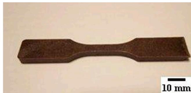
Figure 3. ASTM D638-14 Type V.
