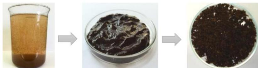
**Figure 3.** The waste wood biomass powder obtained from the coagulated wastewater by centrifugation followed by drying.
