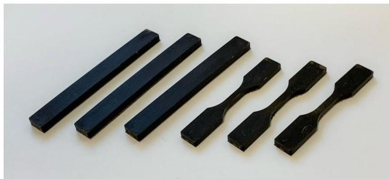
**Figure 9.** The obtained wood–plastic composites for mechanical tests.
