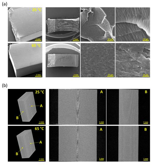
**Figure 4.** Morphology characterization imaging: SEM images showing the surface morphology of the samples on the left and the fracture morphology following the Charpy impact test at various magnifications on the right–(a) and CT images showing a 3D preview of a scanned sample with the scanning directions marked on the left and images showing sections of the internal structure from two sides (views from direction A and B) perpendicular to each other on the right–(b).
