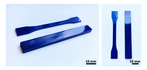
Figure 3. Images of the mechanical test specimens after molding process from different views.
