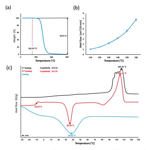
Figure 2. Thermal properties of the PDO granulate: TGA analysis of the thermal degradation -(a), MVR rheological measurement -(b) and DSC curves of the crystallinity and transition temperatures -(c).
