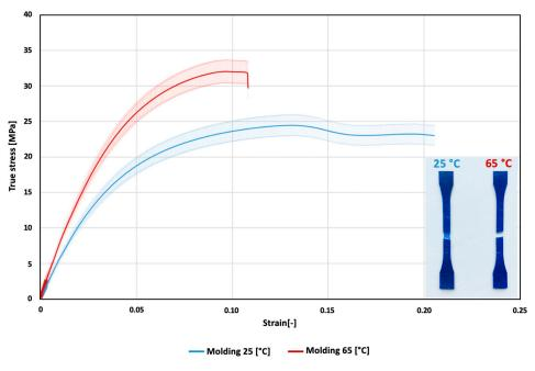
**Figure 6.** Tensile curves of the average values together with standard deviations for the 25  $^{\circ}$ C and 65  $^{\circ}$ C samples.
