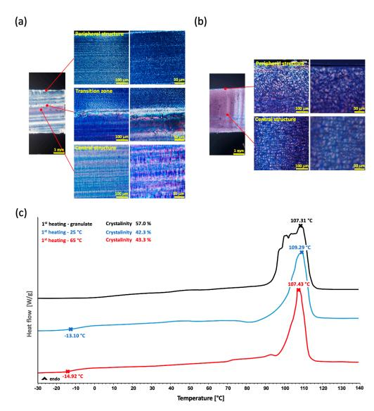
**Figure 5.** Images of the inner structure analysis: POM images of the inner structure for the 25 °C sample–(**a**), POM images of the inner structure for the 65 °C sample–(**b**) and DSC curves of the 1st heatings of both samples–(**c**).
