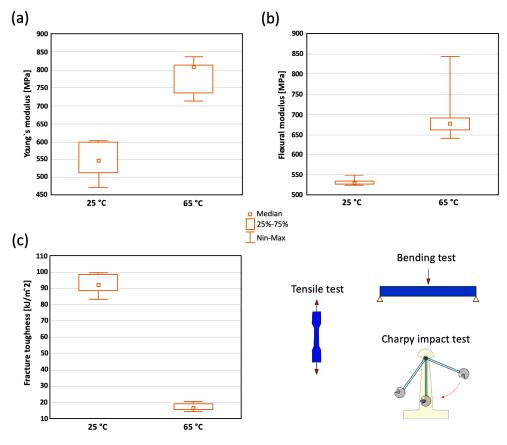
**Figure 7.** Boxplots illustrating the mechanical properties of the 25 °C and 65 °C samples; tensile modulus–(**a**), flexural modulus–(**b**) and fracture toughness–(**c**).
