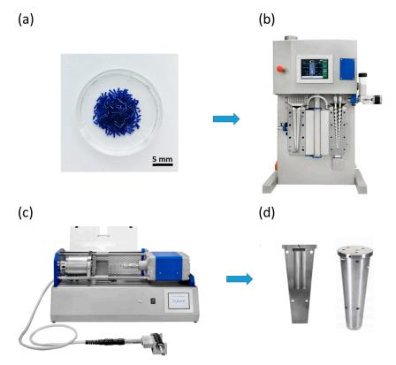
**Figure 1.** Scheme of the micro injection molding processing: PDO granulate–(**a**), twin-screw compounder–(**b**), micro injection machine–(**c**) and injection mold–(**d**).
