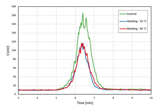
**Figure 8.** GPC chromatograms of the PDO molded samples: control (PDO granulate), molding–25 °C and molding–65 °C.
