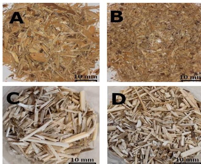
**Figure 1.** Particle size for each layer of the board: (A) industrial particles for the core layer, (B) industrial particles for the surface layers, (C) hemp shives for the core layer, (D) hemp shives for surface layers.
