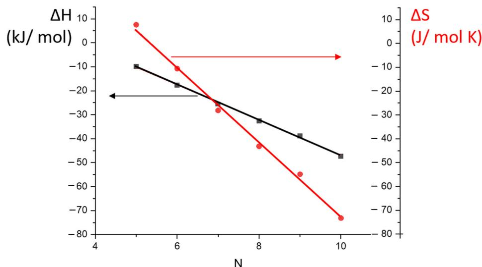
**Figure 5.** Correlation of the enthalpy  $\Delta H$  and entropy  $\Delta S$  of the sorption of n-alkanes during the PM stationary phase with the methylene group number for the n-alkane molecules.
