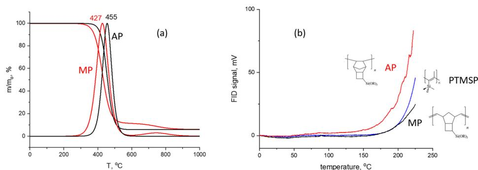
**Figure 2.** TGA curves demonstrating the percentage mass loss of the polymers depending on the temperature (a) and baseline stability under GC conditions of the AP and MP stationary phases and the PTMSP stationary phase (b).
