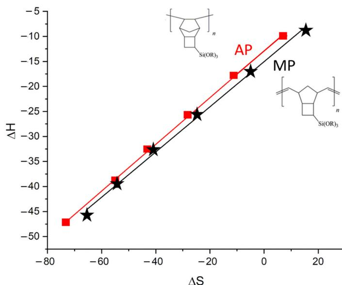
**Figure 6.** Compensation plots for the sorption of n-alkanes during the AM and PM stationary phases.
