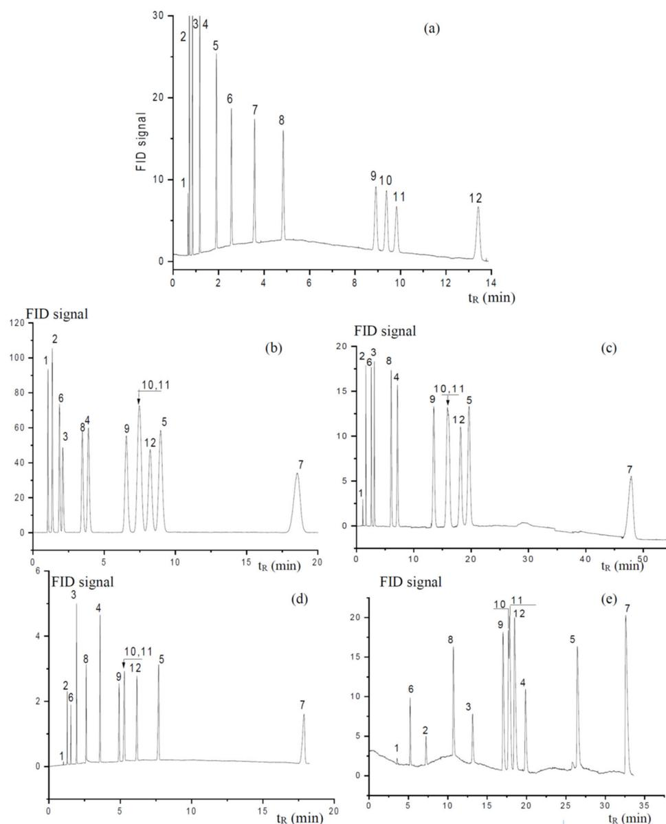
**Figure 3.** Separation of the test mixture during the investigated stationary phases: (a)—PEG 20 M, (b)—AP, (c)—MP, (d)—SE-30, (e)—PTMSP. Test mixture: 1—n-pentane, 2—n-hexane, 3—n-heptane, 4—n-octane, 5—n-nonane, 6—benzene, 7—n-decan, 8—toluene, 9—ethylbenzene, 10—p-xylene, 11—m-xylene, 12—o-xylene. Separation conditions were as follows: column temperature 40 °C, isothermal for (a–d) chromatograms, and 130 °C for (e) chromatogram, carrier gas helium, inlet pressure 70 kPa.
