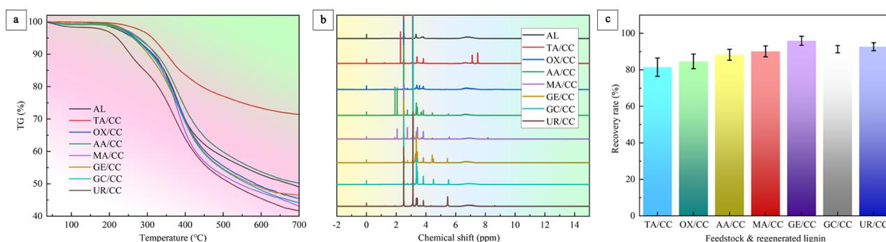
**Figure 2.** (a) TGA curves of AL, TA/CC, OX/CC, AA/CC, MA/CC, GE/CC, GC/CC, and UR/CC; (b) <sup>1</sup>H NMR spectra of AL, TA/CC, OX/CC, AA/CC, MA/CC, GE/CC, GC/CC, and UR/CC; (c) DES recovery for TA/CC, OX/CC, AA/CC, MA/CC, GE/CC, GC/CC, and UR/CC.
