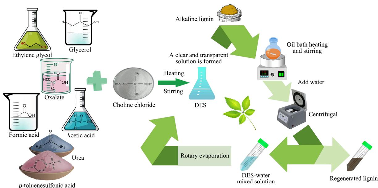
**Scheme 1.** Process flow chart of lignin degradation and DES recovery.
