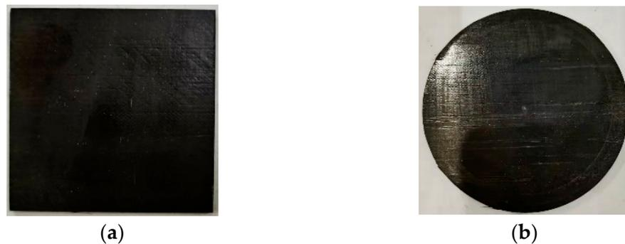
**Figure 2.** Square and circular CFRP specimens. (a) Square CFRP specimens; (b) circular CFRP specimens.
