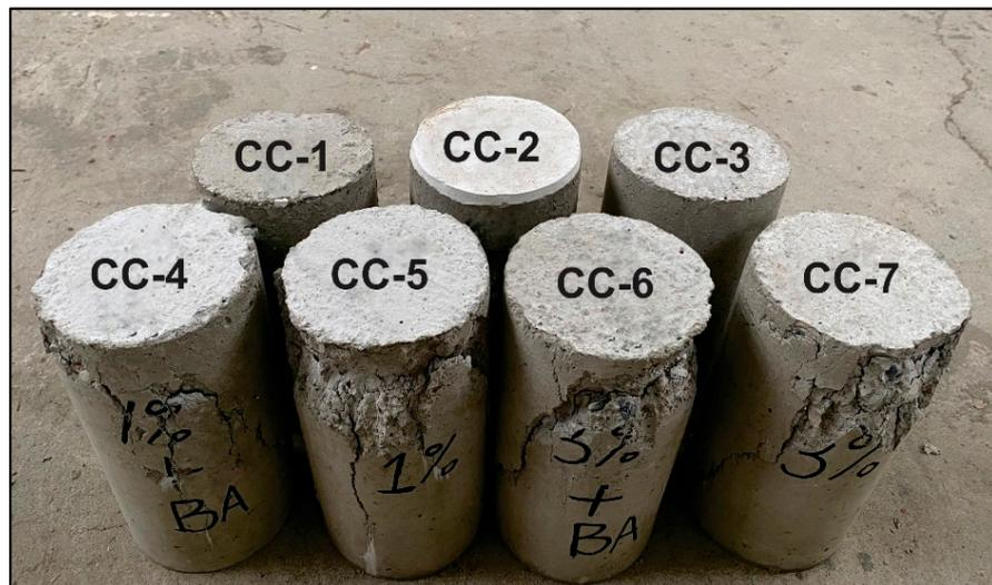
**Figure 7.** Photograph of cylindrical concrete specimens after applied load.
