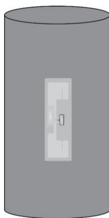
Figure 6. Schematic diagram of the 3D-printed protection of smart sensor tag embedded in cylindrical concrete.
