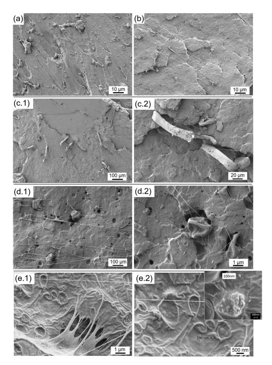
**Figure 8.** FESEM images of the fracture surface of the PLA-MCO-silk composites: (a) Neat PLA, (b) PLA-MCO, (c.1,c.2) PLA-MCO-CS, (d.1,d.2) PLA-MCO-SFM, and (e.1,e.2) PLA-MCO-SFN at different magnifications.
