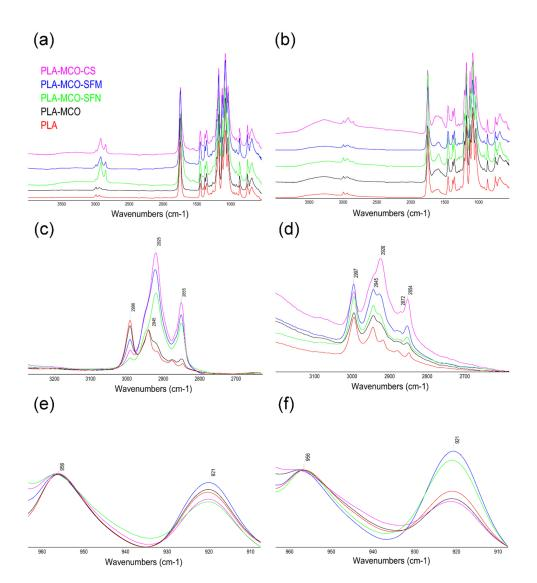
**Figure 10.** Comparative evolution of the ATR-FTIR spectra along the incubation at composting conditions: Full spectra of the composites at days 1 (**a**) and 30 (**b**). Detail of the spectral region  $3200-2700 \text{ cm}^{-1}$ , at days 1 (**c**) and 30 (**d**). Detail of the spectral region  $960-910 \text{ cm}^{-1}$ , at days 1 (**e**) and 30 (**f**).
