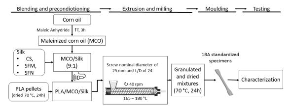
Figure 3. Flow chart of the process used for the preparation of PLA-MCO-Silk composites.
