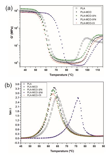
**Figure 5.** Effect of the temperature on the storage modulus (G') (**a**) and damping factor (*tan*  $\delta$ ) (**b**) of neat PLA, plasticized PLA, and PLA-Silk formulations.
