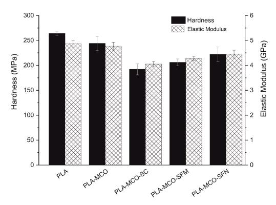
Figure 4. Hardness and elastic modulus acquired for each formulation by nanoindentation technique.
