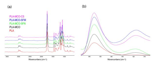
**Figure 6.** ATR-FTIR spectra of the Silk-MCO-PLA composites. (**a**) Full spectra of the composites. (**b**) Selected region of the spectra used to measure the relative crystallinity of PLA.
