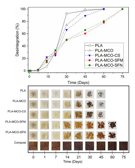
**Figure 9.** Photographic registry of the Disintegration of PLA and different PLA-composites, containing MCO and silk fillers, under controlled composting conditions.
