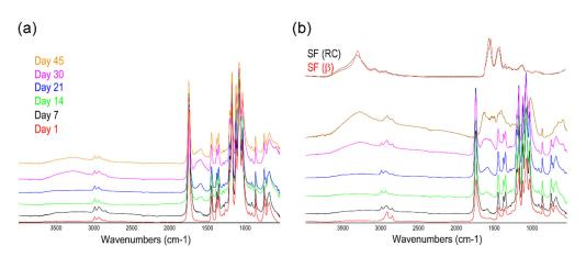
**Figure 11.** Comparative evolution of the ATR-FTIR spectra along the incubation at composting conditions: Full spectra of the PLA from day 1 to 45 (**a**) and PLA-MCO-CS from day 1 to 45 (**b**). Pure fibroin in random coil (RC) or  $\beta$ -sheet ( $\beta$ ) conformation is inserted for comparison purposes.
