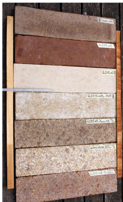
**Figure 31.** Sawdust-based panels of different wood species. Reprinted with permission from ref. [74].
