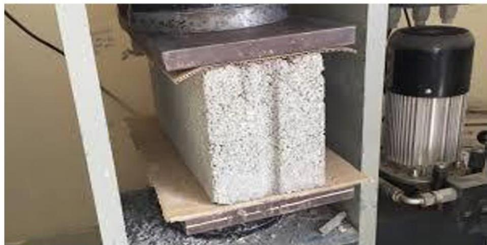
Figure 23. Compression testing of PS/cement composite material. Reprinted with permission from ref. [65].
