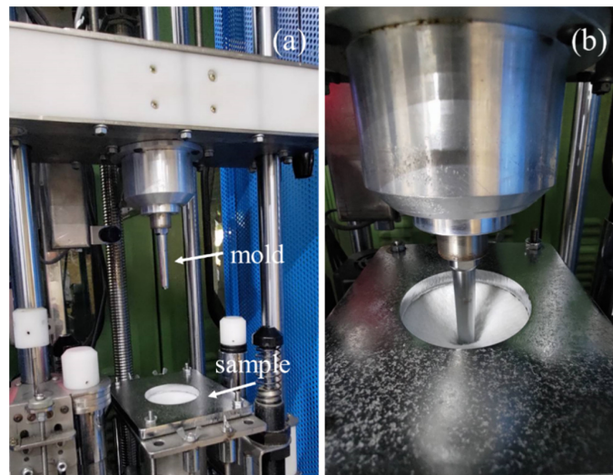
Figure 4. (a) Schem of dynamic impact strength test; (b) Test the situation.
