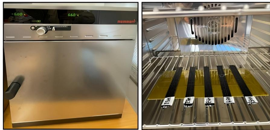
**Figure 2.** An air-circulated oven for hot temperature treatment.
