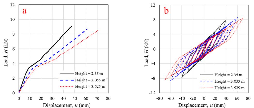
**Figure 13.** Horizontal in-plane lateral load versus displacement from validated numerical modeling with different log-wall heights under (a) monotonic loading; (b) cyclic loading.
