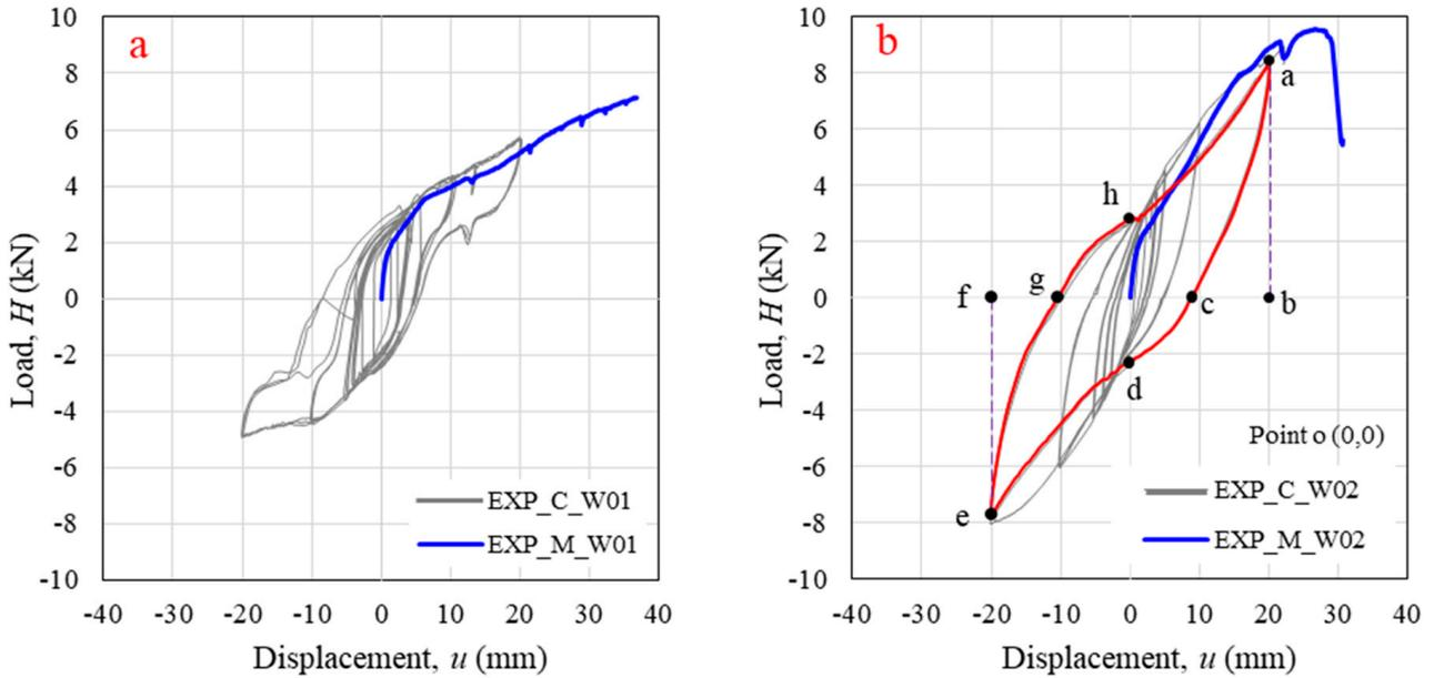
**Figure 6.** Horizontal in-plane lateral load versus displacement relationship (at DT A) under monotonic (EXP\_M) and cyclic (EXP\_C) loading for (a) Specimen W01; (b) Specimen W02.
