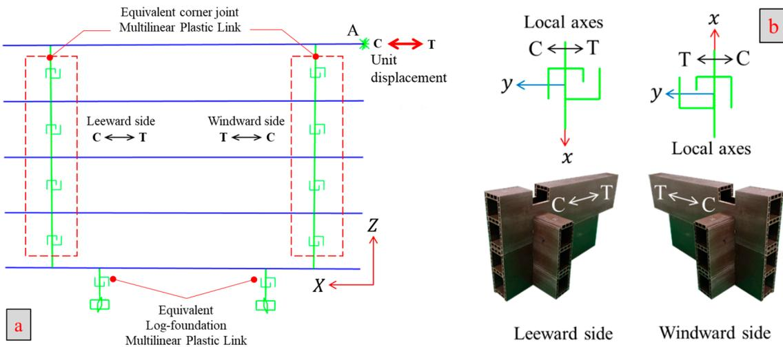
**Figure 10.** Finite element modeling schematic for WPVC composite log-wall: (a) Overall view; (b) Details of corner joints on leeward and windward sides.
