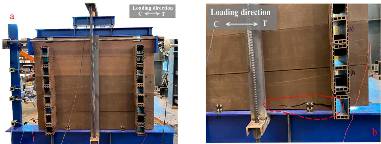
**Figure 8.** WPVC composite log-wall specimen (W01) under compressive loading: (a) Overall deformed shape; (b) Separation between first main log-member and support.
