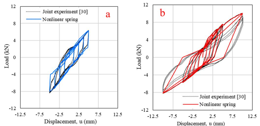
**Figure 9.** Nonlinear spring calibration with previous experiment for (a) Standard half-lapped corner joint (CJ-SHL); (b) Angle bracket first log-foundation connection (LF-AB).
