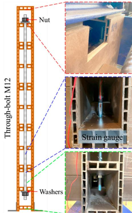
Figure 3. Detail of through-bolt connection for specimen W02.
