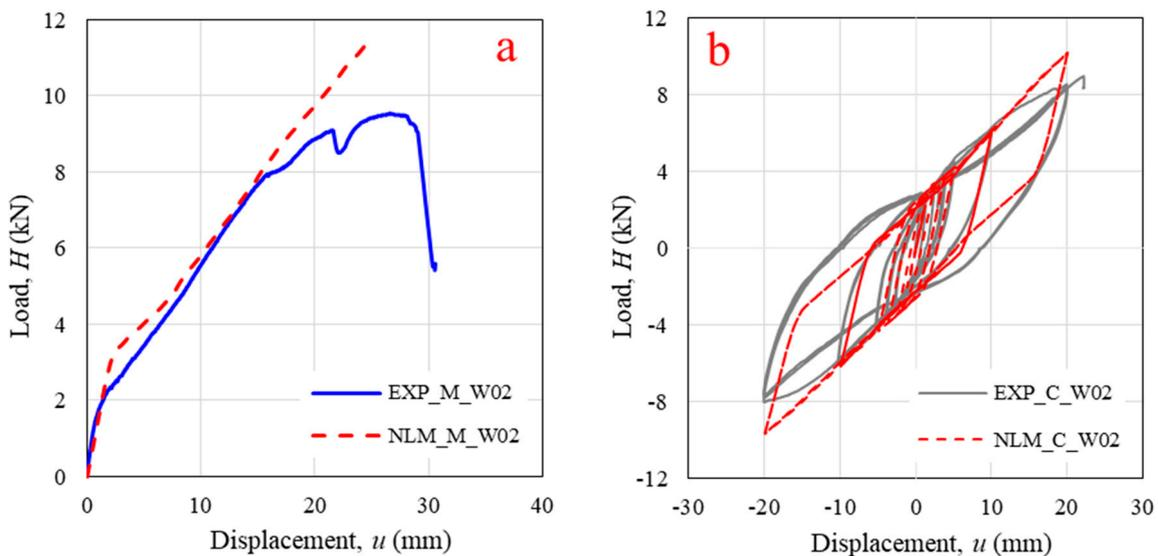
**Figure 11.** Comparison of experimental (EXP) and finite element model (FEM) results for specimen W02 under (a) monotonic loading; (b) cyclic loading.
