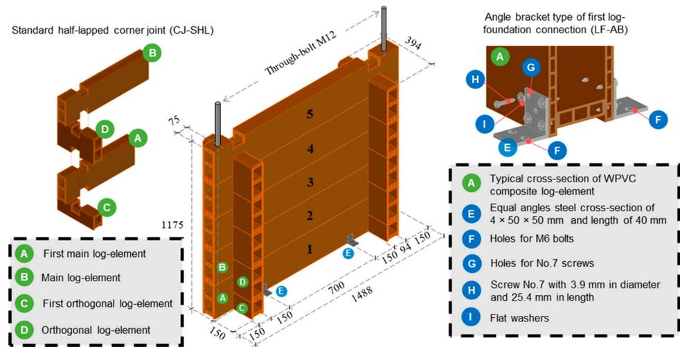
Figure 2. Layout of full-scale WPVC composite log-wall specimens W01 and W02.
