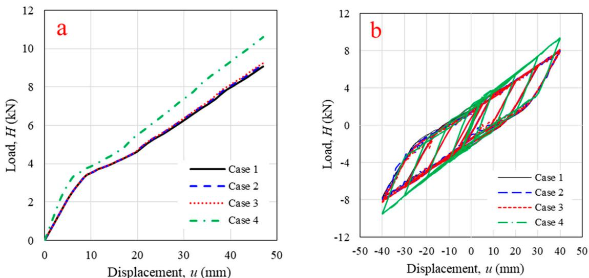
**Figure 15.** Horizontal in-plane lateral load versus displacement from validated numerical modeling with different log-foundation connection configurations under (a) monotonic loading; (b) cyclic loading.
