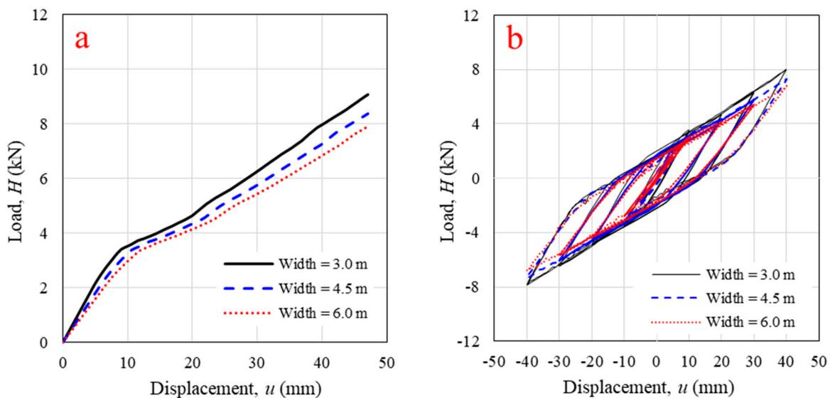
**Figure 14.** Horizontal in-plane lateral load versus displacement from validated numerical modeling with different log-wall widths under (a) monotonic loading; (b) cyclic loading.
