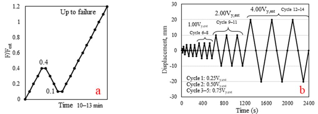
**Figure 5.** Horizontal in-plane loading protocol for (a) monotonic; (b) cyclic loading.
