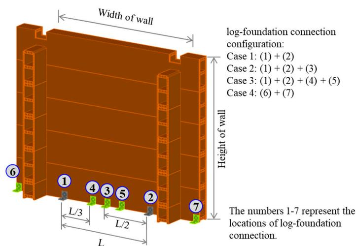
**Figure 12.** Schematic of WPVC composite log-wall for parametric studies.
