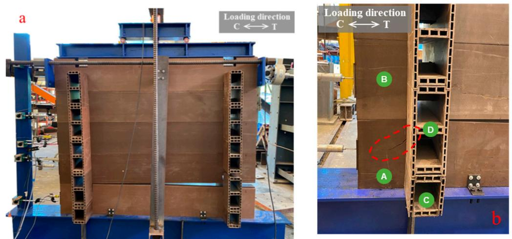
**Figure 7.** WPVC composite log-wall specimen (W01) under compressive loading: (a) Overall deformed shape; (b) Tearing of first main log-member (log A).
