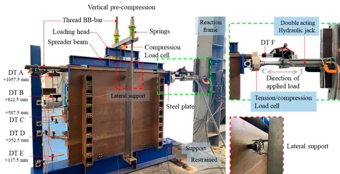
**Figure 4.** In-plane lateral load experimental setup (instrument positions and lateral support) performed on WPVC composite log-wall (C is compressive direction and T is tensile direction).
