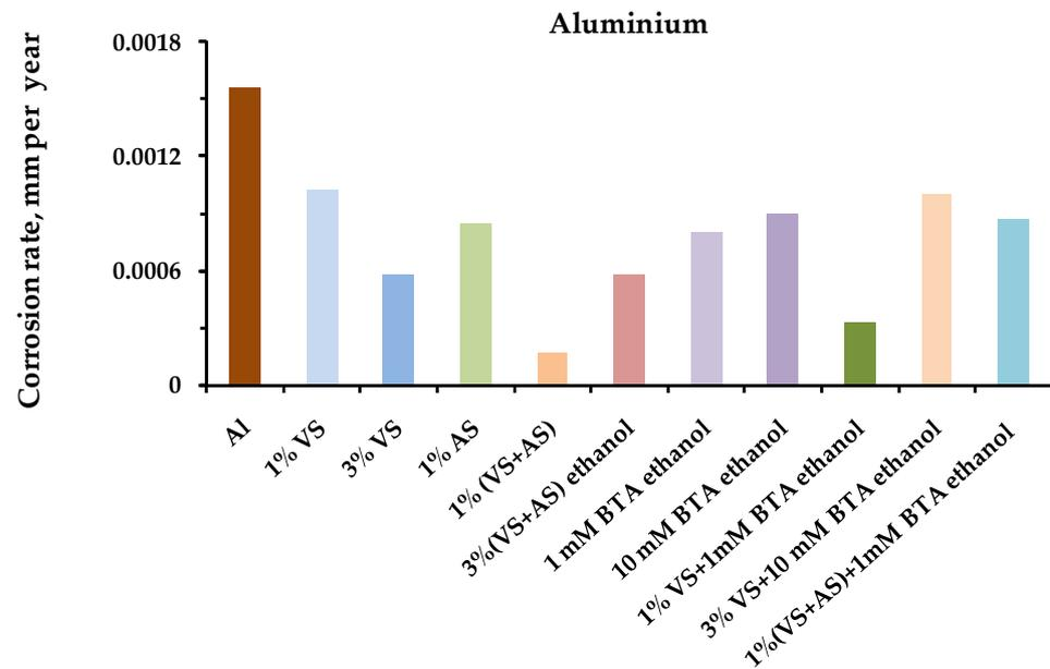
**Figure 4.** Atmospheric corrosion rates (mm per year) of **aluminium** modified by organosilane-based compositions. Full-scale, one-year corrosion tests, carried out in an urban atmosphere. Gravimetric assessment of corrosion magnitude.
