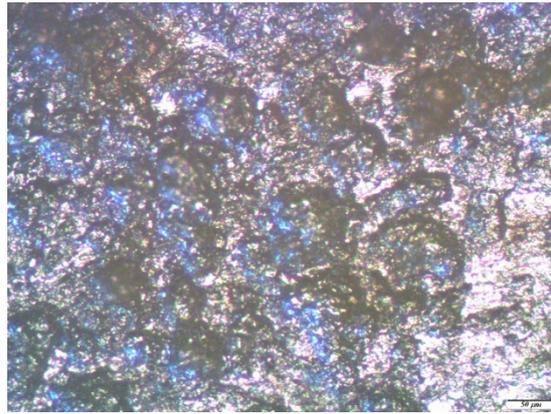
**Figure 13.** Micrograph of the surface area of an unmodified steel sample after the removal of the corrosion products.
