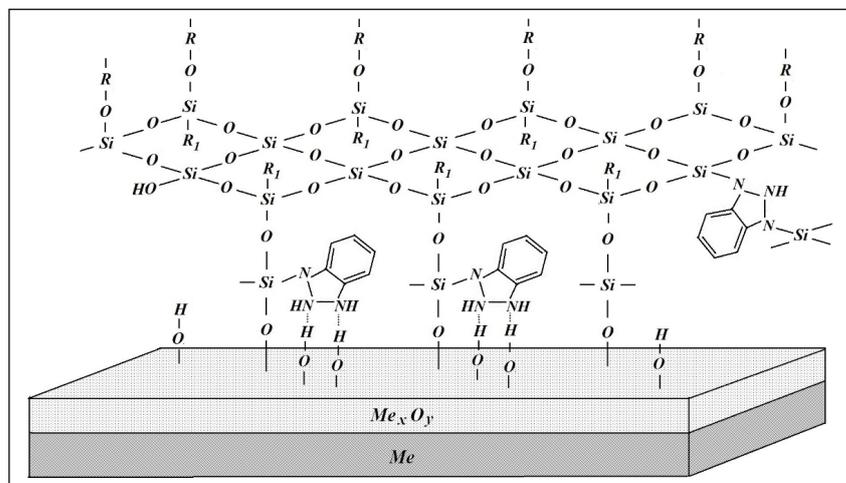
**Figure 6.** Scheme of the structure of the interface metal/siloxane–azole layer.
