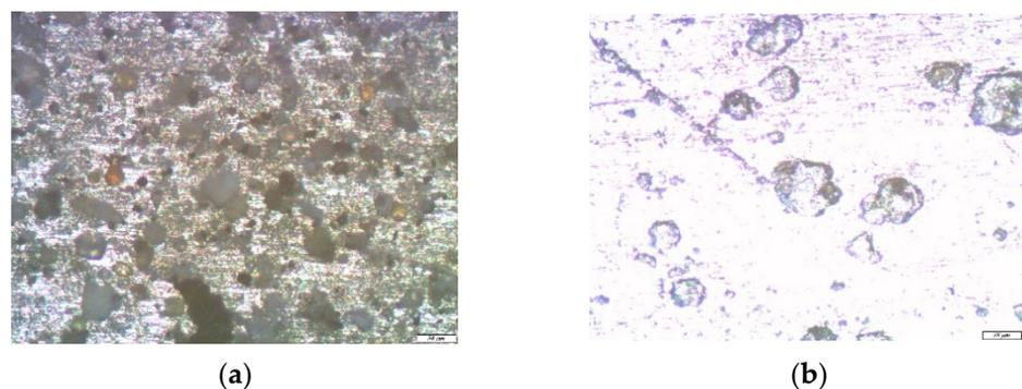
**Figure 8.** Micrographs of the surface area of the zinc sample, pre-modified with a 1% VS solution, after conducting full-scale, one-year natural tests in an urban atmosphere: (a) immediately after testing but before the removal of the corrosion products; and (b) after the removal of the corrosion products.
