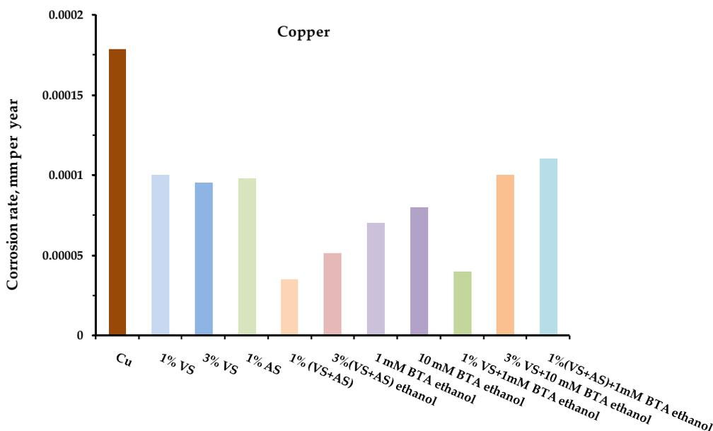
**Figure 2.** Atmospheric corrosion rates (mm per year) of **copper** modified by organosilane-based compositions. Full-scale, one-year corrosion tests, carried out in an urban atmosphere. Gravimetric assessment of corrosion magnitude.
