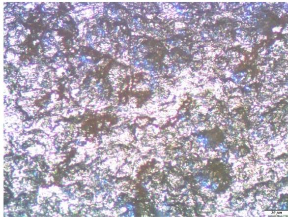
**Figure 14.** Micrograph of the surface area of a carbon steel sample, modified with a 1% VS water solution or 3% VS water solution, after conducting full-scale, one-year natural corrosion tests in an urban atmosphere and removing the corrosion products.
