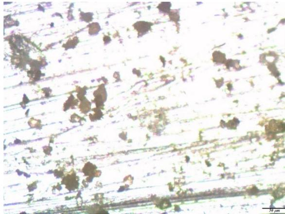
**Figure 11.** Micrograph of the surface area of an unmodified aluminum sample after conducting full-scale, one-year tests in an urban atmosphere, after the removal of the corrosion products.
