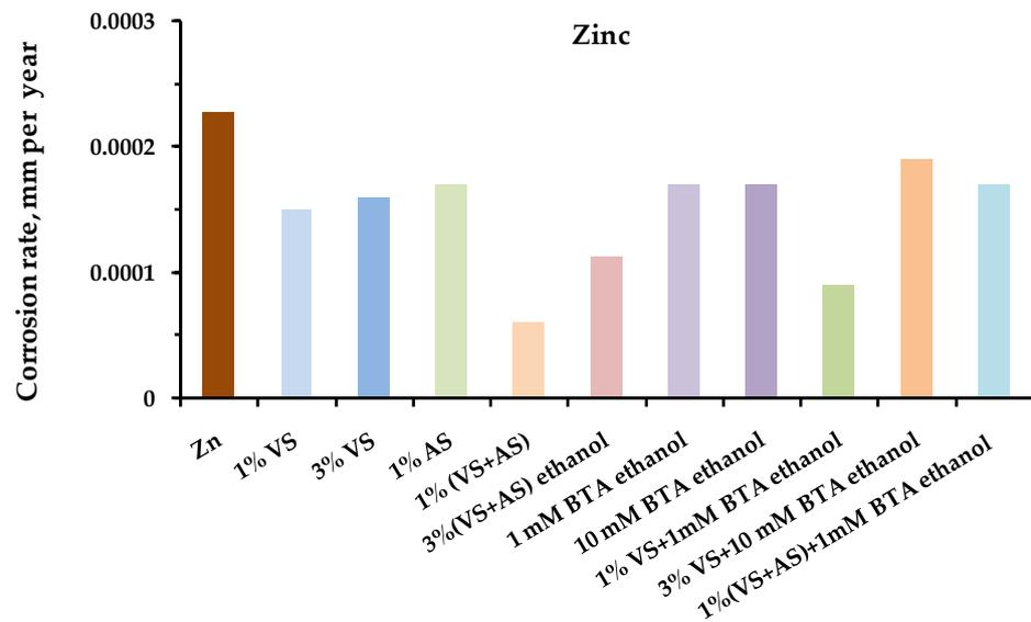
**Figure 3.** Atmospheric corrosion rates (mm per year) of **zinc** modified by organosilane-based compositions. Full-scale, one-year corrosion tests, carried out in an urban atmosphere. Gravimetric assessment of corrosion magnitude.
