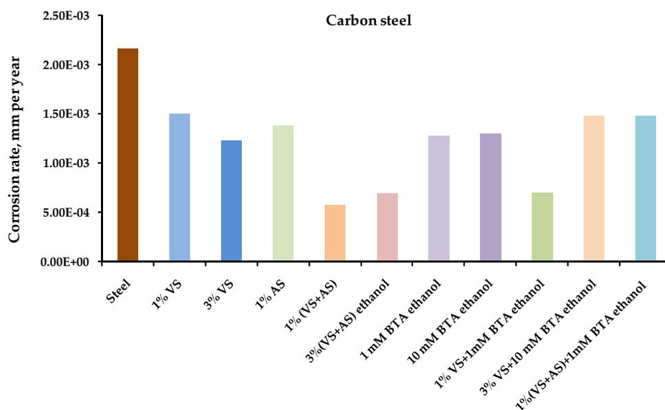
**Figure 1.** Atmospheric corrosion rates (mm per year) of **carbon steel** modified by organosilane-based compositions. Full-scale, one-year corrosion tests, carried out in an urban atmosphere. Gravimetric assessment of corrosion magnitude.
