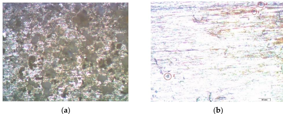
**Figure 9.** Micrographs of the surface area of a zinc sample pre-modified with a solution containing a mixture of [1% VS + 1% AS] after conducting full-scale, one-year natural tests in an urban atmosphere: (a) immediately after the tests but before the removal of the corrosion products; and (b) after the removal of the corrosion products. Optical magnification of 10 $\times$ , with defects highlighted in red.
