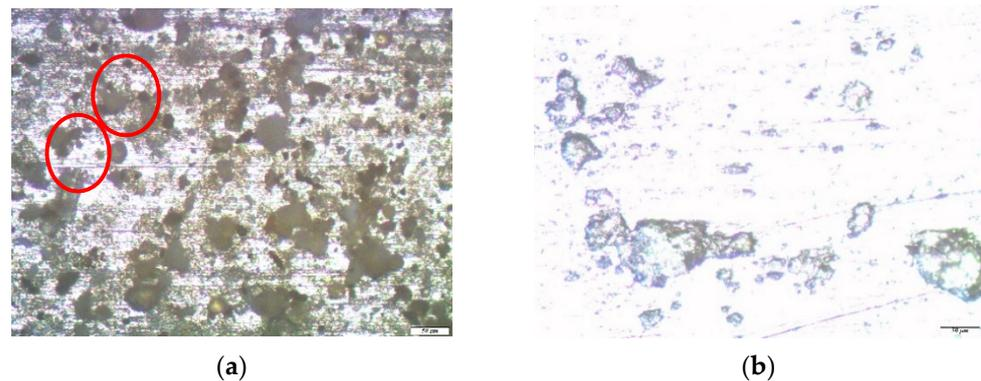
**Figure 7.** Micrographs of the surface area of an unmodified zinc sample after conducting one-year field tests in an urban atmosphere: (a) immediately after testing but before the removal of corrosion products, with hemispherical pitting marked in red; and (b) after the removal of corrosion products.
