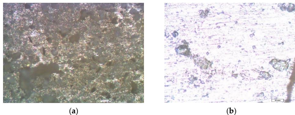
**Figure 10.** Micrographs of the surface area of a zinc sample pre-modified with a solution containing a mixture of [1% VS + 1 mM BTA], after conducting full-scale, one-year natural tests in an urban atmosphere: (a) immediately after testing but before the removal of the corrosion products; and (b) after the removal of the corrosion products. Optical magnification of 10 $\times$ .
