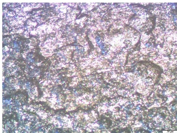
**Figure 15.** Micrograph of the surface area of a carbon steel sample, modified with solution of a mixture [1% VS + 1% AS], after conducting full-scale, one-year natural corrosion tests in an urban atmosphere and removing the corrosion products.
