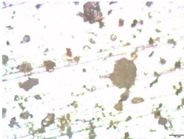
**Figure 12.** Micrograph of the surface area of an aluminum sample modified with a solution of a mixture of [1% VS + 1 mM BTA], after conducting full-scale, one-year natural tests in an urban atmosphere and removing the corrosion products.
