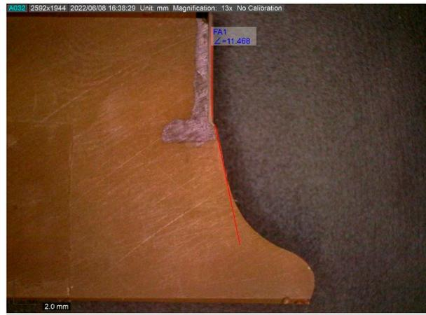
**Figure 5.** Estimation of angular direction of crack growth using a digital microscope.
