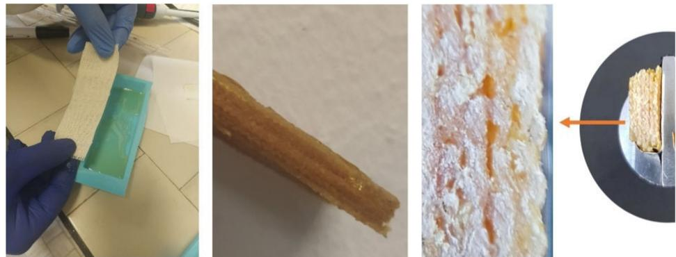
**Figure 6.** Preparation by hand-layup and cured composite laminate based on AEHO resin and hemp fibres.
