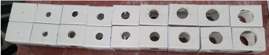
**Figure 2.** Specimens with different opening sizes.
