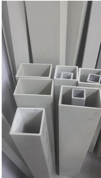
**Figure 1.** Pultruded GFRP profiles.
