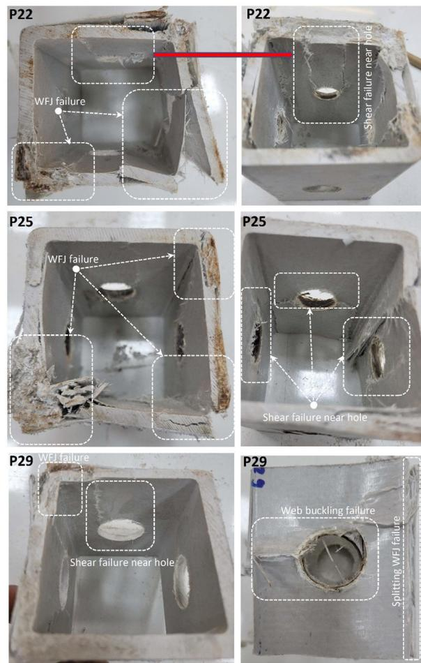
Figure 6. Damage analyses of P22, P25, and P29.
