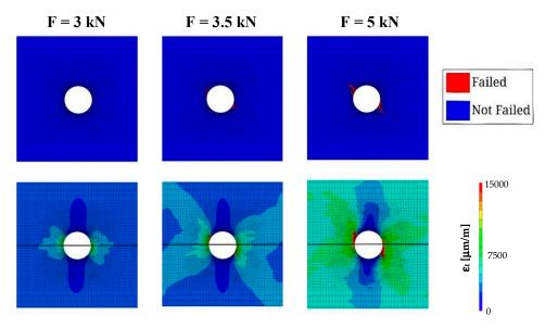
**Figure 5.** Matrix damage (IFF) and first principal strain ( $\varepsilon_I$ ) pattern progression.
