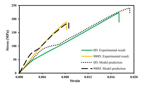
**Figure 6.** Stress–strain plot: experimental results and prediction of the effects of the seawater exposure for 0 and 900 immersion days.
