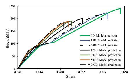
**Figure 10.** Stress–strain plot: model prediction of the effects of the seawater exposure for different immersion time.
