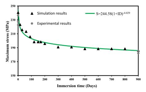
**Figure 11.** Maximum stress against immersion time: numerical predictions and experimental results for 0 and 900 immersion days.
