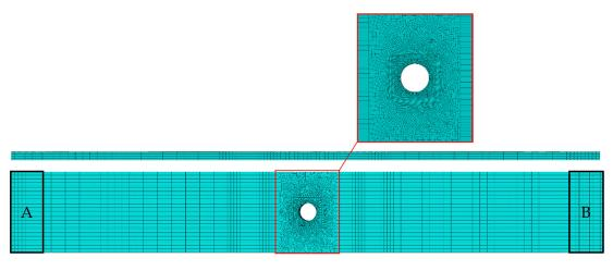
Figure 3. Finite element mesh used in the numerical simulations.
