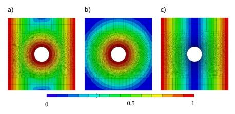
**Figure 12.** Seawater concentration after 900 immersion days with: (**a**) all permeable surfaces; (**b**) impermeable lateral surfaces; (**c**) impermeable hole surface.
