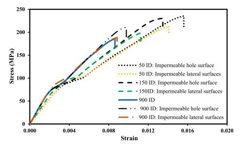
Figure 13. Prediction of the maximum stress for different impermeable surfaces.
