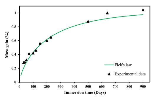
**Figure 1.** Comparison of Fick's law for predicting the seawater absorption and the experimental results for the tested laminate.
