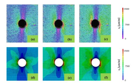
**Figure 4.** Comparison between the first principal strain ( $\varepsilon_1$ ) fields obtained experimentally and numerically. Images a, b and c correspond to the experimental results, and the remaining ones to the simulations with the application of Puck's failure theory; the images (**a**,**d**), (**b**,**e**) and (**c**,**f**) correspond to loads of 4.3 kN, 4.875 kN and 5.5 kN, respectively.
