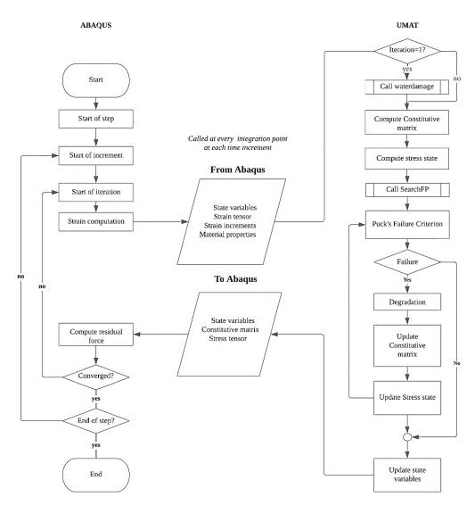
Figure 2. Algorithm of the 3D-FE iterative procedure developed in this study.
