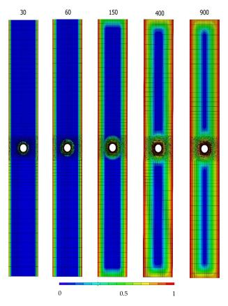
Figure 9. Prediction of the concentration of seawater after 30, 60, 150, 400 and 900 days of immersion.
