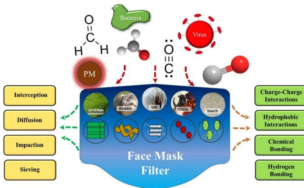
**Figure 5.** Principal biopolymers used in filtration applications, and their interaction mechanisms with the micro-organisms (virus and bacteria) and other toxic particles. Reproduced with permission from [80].
