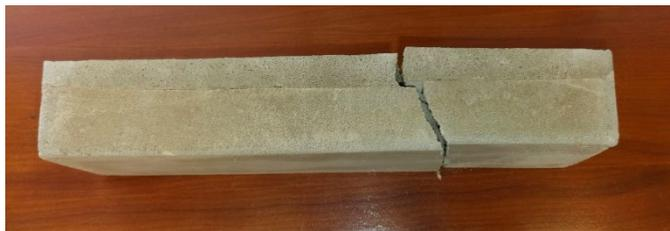
**Figure 26.** Detail of delamination-specimen 22030420.
