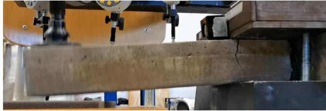
**Figure 24.** Collapse of specimen 19030420 after load test (composite FC and CC) without delamination.
