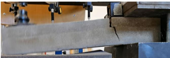
**Figure 27.** Delamination of specimen 24030420 after load test (composite FC and CC).
