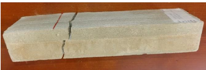
**Figure 28.** Detail of delamination-specimen 24030420.
