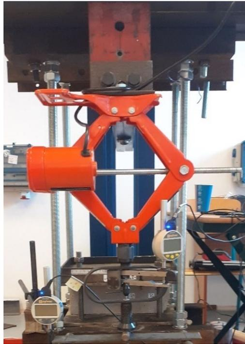
**Figure 5.** Mechanism used to introduce the load into the specimen.
