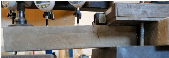
**Figure 25.** Delamination of specimen 22030420 after load test (composite FC and CC).
