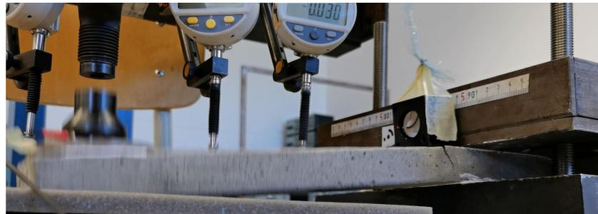
Figure 11. Collapse of the CC specimen 5200420.
