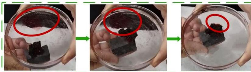
**Figure 7.** Oil–water separation using the MFA @ PDMS sponge.
