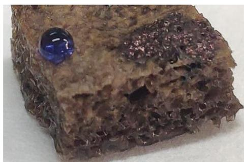
**Figure 6.** Hydrophobic Properties of MFA@PDMS sponge.
