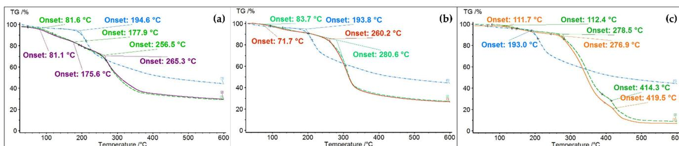
**Figure 6.** Thermograms of: (a) chitosan–cellulose–dye film (violet), chitosan–cellulose film (green), and dye (blue); (b) chitosan–starch–dye film (green), chitosan–starch film (red), and dye (blue); (c) chitosan–PVA–dye film (green), chitosan–PVA film (orange), and dye (blue).
