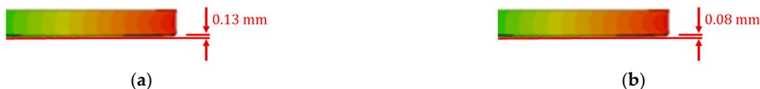
**Figure 7.** Numerically predicted warpage for 3D printed samples at different layer heights: (a) 0.15 mm, (b) 0.10 mm.
