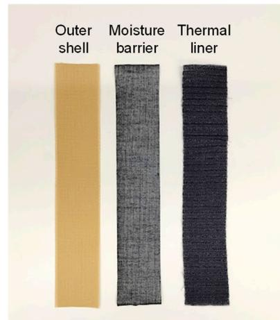
**Figure 1.** Example of firefighters' protective clothing fabrics (Sample A).
