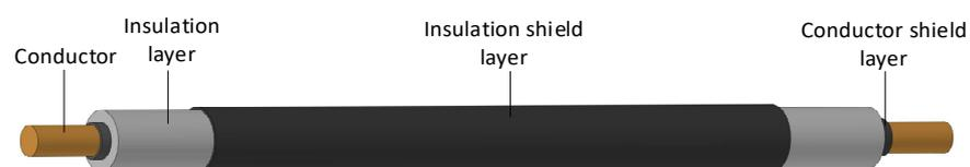
Figure 1. The cable sample.
