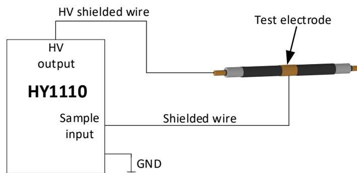
**Figure 2.** The cable capacitance and dielectric loss factor measurement device.
