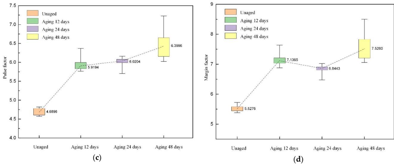
**Figure 10.** The distribution of dimensionless parameters in the time domain. (a) Waveform factor; (b) crest factor; (c) pulse factor; (d) margin factor.
