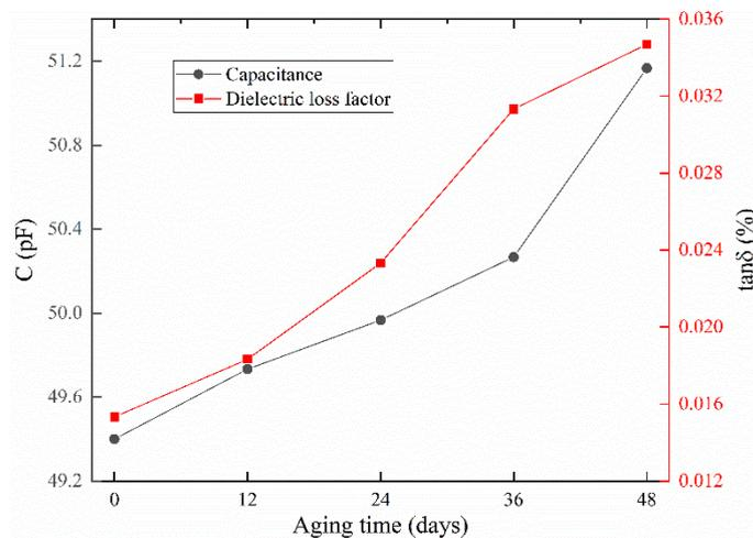
**Figure 4.** The changes in capacitance and dielectric loss factor of cable sample with aging time.
