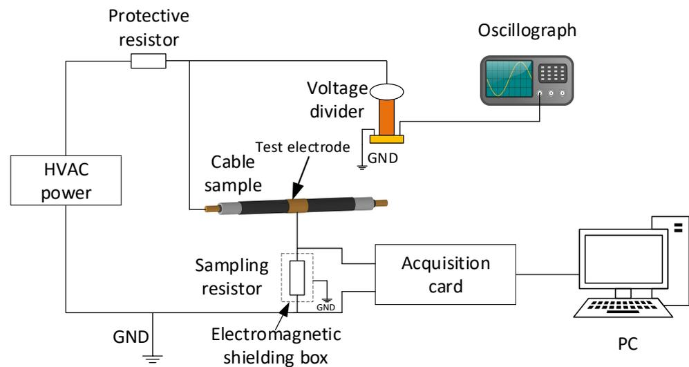
**Figure 3.** The AC leakage current test experimental setup.
