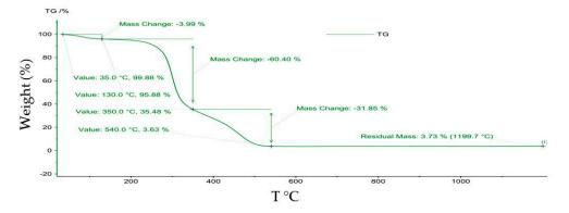
Figure 9. TG curve of maize stalk after adsorption process.
