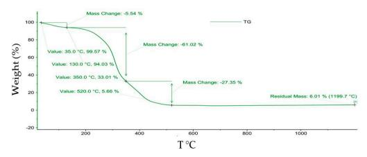
Figure 8. Curve of TG regarding maize stalk before adsorption process.
