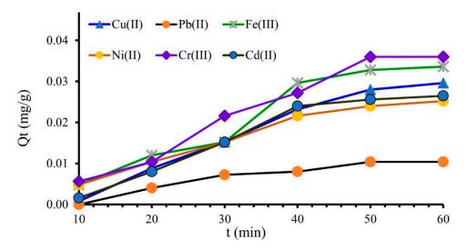
**Figure 2.** Influence of contact time on the retention of metal ions onto MS mass, 0.04 L of  $M^{X+}$  (Ci = 0.5 mg/L), contact time 10–60 min, 0.5 g MS, 175 rpm (25  $\pm$  2 °C), pH = 4.2.
