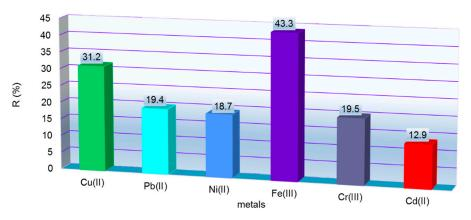
**Figure 6.** Removal of  $M^{X+}$  from tannery wastewaters onto MS mass. Experimental conditions: 0.04 L of tannery wastewaters that contained  $M^{X+}$  (Ci = 0.218 mg  $Cu^{2+}/L$ , 0.618 mg  $Pb^{2+}/L$ , 1.073 mg  $Ni^{2+}/L$ , 0.163 mg  $Cd^{2+}/L$ , 1006 mg  $Cr^{3+}/L$  and 0.633 mg  $Fe^{3+}/L$ ), contact time 60 min, 175 rpm, 0.5 g MS, pH = 4.3.
