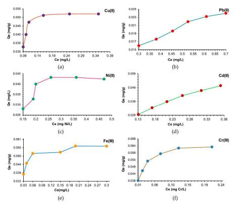
**Figure 3.** Effect of M<sup>X+</sup> initial concentration on the adsorption capacity of MS. Experimental conditions:  $Ci = 0.5-1 \text{ mg/L M}^{X+}$ , contact time 60 min, 175 rpm (25 ± 2 °C), 0.5 g of MS, pH = 4.2.
