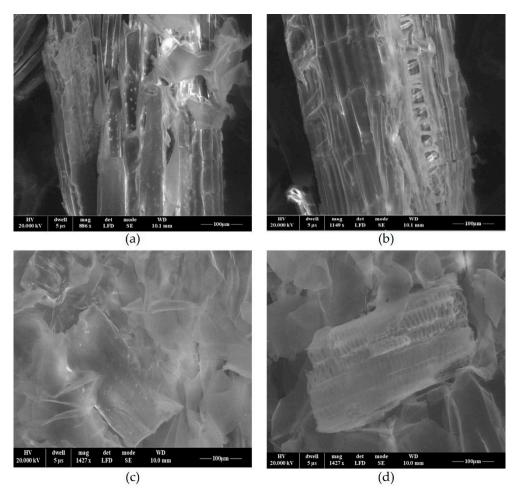
**Figure 10.** SEM images of MS at  $1147 \times (\mathbf{a})$ ,  $886 \times (\mathbf{b})$ ,  $1427 \times (\mathbf{c},\mathbf{d})$  magnification before  $(\mathbf{a},\mathbf{b})$  and after  $(\mathbf{c},\mathbf{d})$  adsorption.
