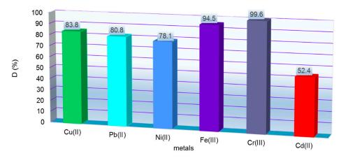
**Figure 7.** Desorption of M<sup>X+</sup> from MS after adsorption process.
