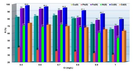
**Figure 4.** Removal of  $M^{X+}$  from simulated textile wastewater onto MS. Experimental conditions: Ci=0.5-1 mg/L  $M^{X+}$ , contact time 60 min, 175 rpm, 0.5 g MS, pH = 4.2.
