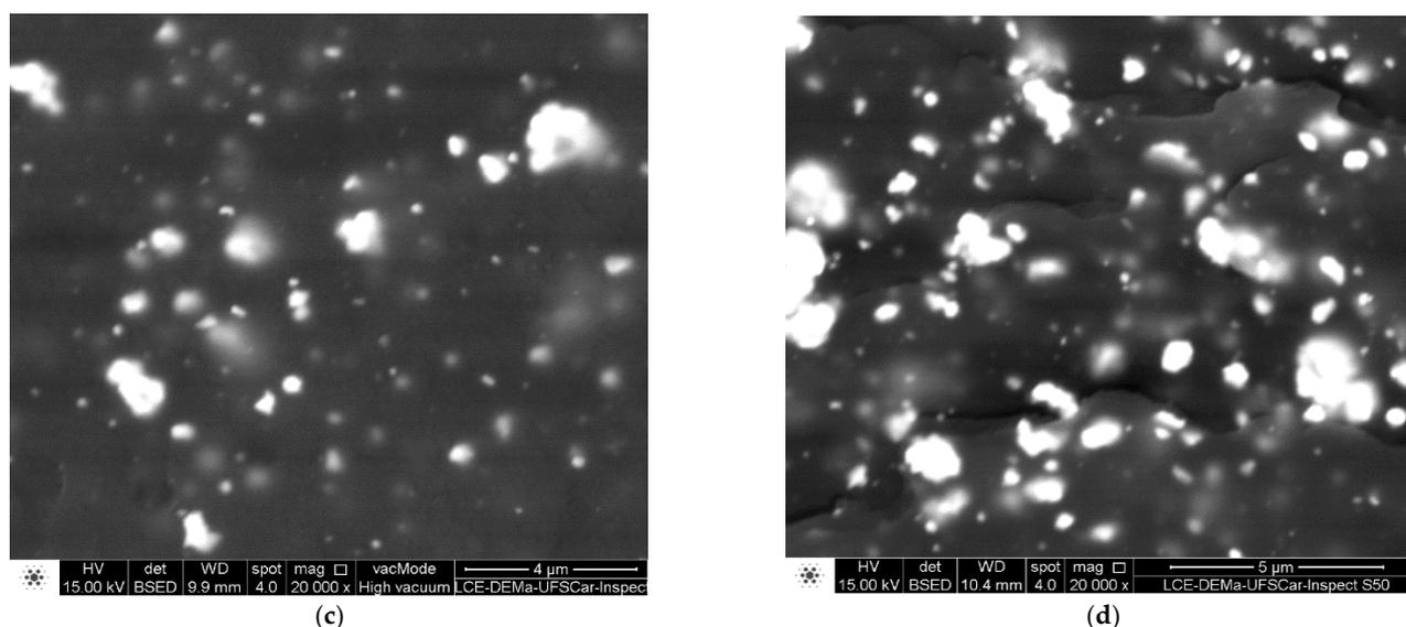
**Figure 6.** SEM images of fractured surfaces of extruded composites: (a) and (c) SNaPZT3<sup>e</sup>; (b) and (d) SNaPZT5<sup>e</sup> (superscript “e” corresponds to extruded material).
