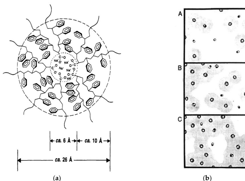
**Figure 1.** Schematic representation of the (a) region of restricted mobility surrounding a multiplet and (b) morphologies of random ionomers at different ion contents: (A) low, (B) intermediate and (C) high ion content. Adapted from Ref [2]. Reprinted with permission from A new multiplet-cluster model for the morphology of random ionomers. A. Eisenberg, B. Hird, and R. B. Moore.
