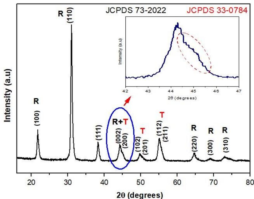
**Figure 4.** Pattern of diffraction of X-ray for PZT particles obtained via Pechini's method, highlighting the typical superposition due to the coexistence of tetragonal (T) (JCPDS file n° 33-0784) and rhombohedral (R) (JCPDS file n° 73-2022) phases at the morphotropic phase boundary region.
