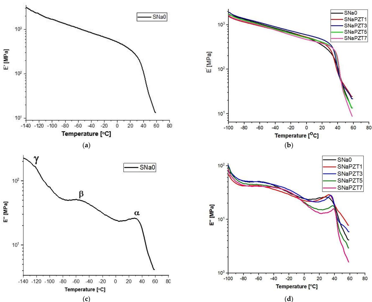
**Figure 11.** DMA curves: (a)  $E'$  for SNa0 film; (b)  $E'$  for different SNaPZT# films; (c)  $E''$  for SNa0 film (with  $\alpha$ ,  $\beta$  and  $\gamma$  relaxations); (d)  $E''$  for different SNaPZT# films.
