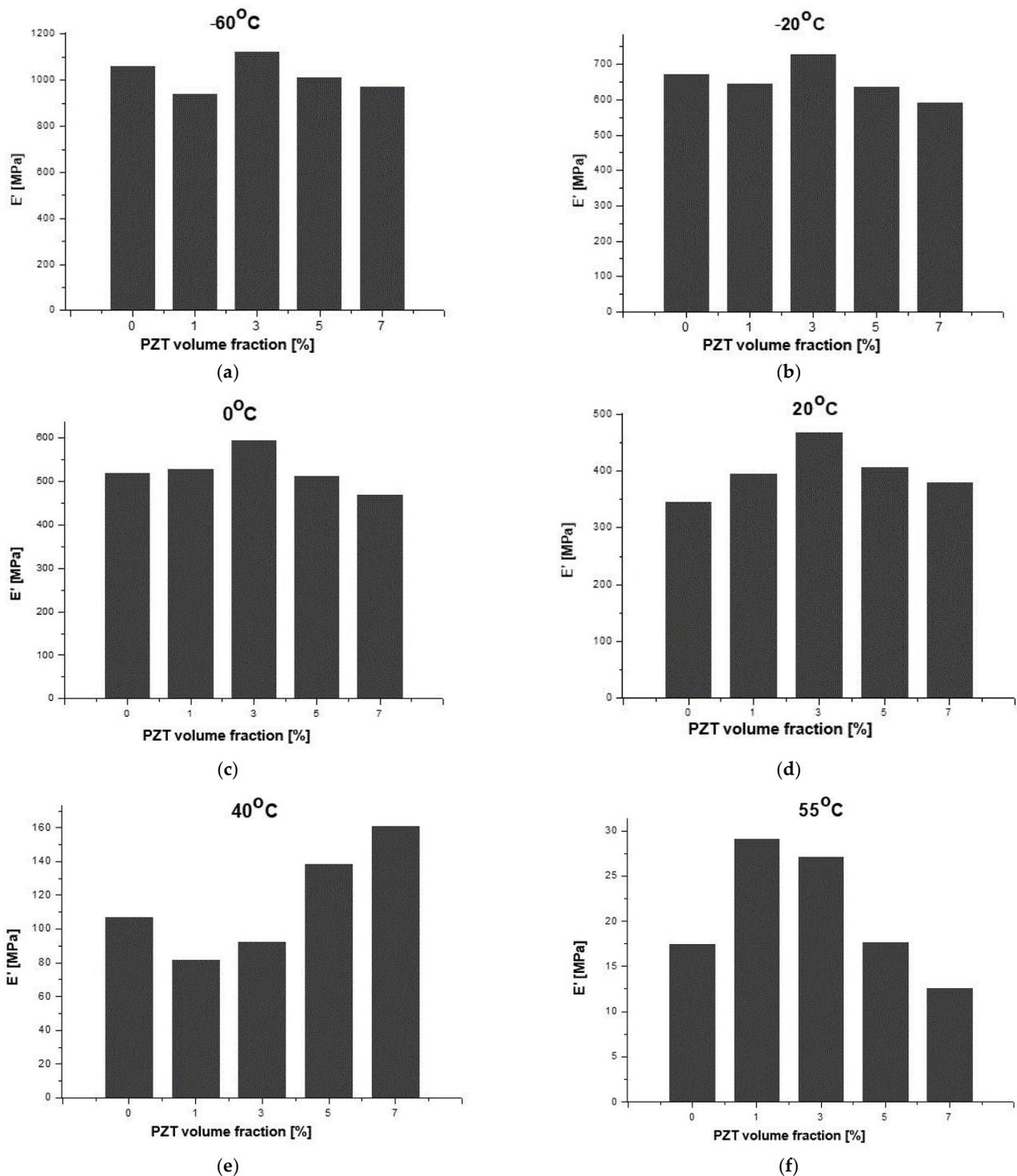
**Figure 12.** Qualitative evaluation of storage modulus ( $E'$ ) of SNa0 and SNaPZT# films at different values of temperature: (a)  $-60^{\circ}\text{C}$ , (b)  $-20^{\circ}\text{C}$ , (c)  $0^{\circ}\text{C}$ , (d)  $20^{\circ}\text{C}$ , (e)  $40^{\circ}\text{C}$  and (f)  $55^{\circ}\text{C}$ .
