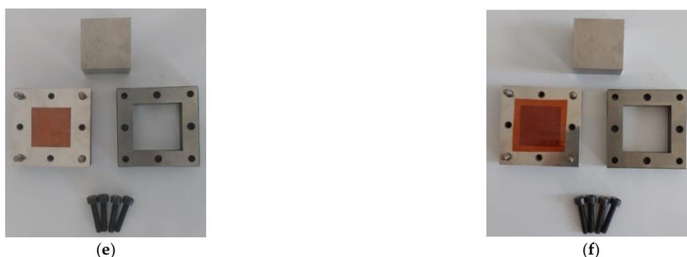
**Figure 2.** Mold used for the manufacturing process of flexible composite films: (a) and (b) the design; (c) assembled mold; (d) mold parts; (e) and (f) Kapton® films used during the process.
