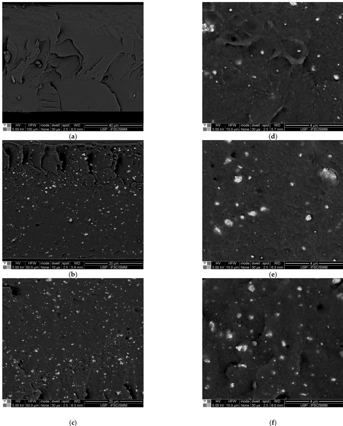
**Figure 7.** SEM images of fractured surfaces of films: (a) SNa0; (b,d) SNaPZT3; (c,e) SNaPZT5; and (f) SNaPZT7.
