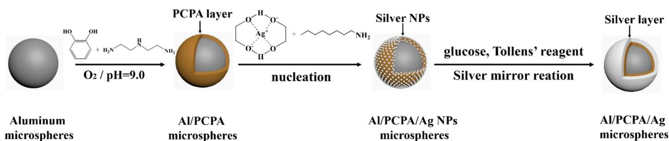
**Scheme 1.** Schematic diagram of the preparation steps for the fabrication of silver-coated aluminum microspheres.
