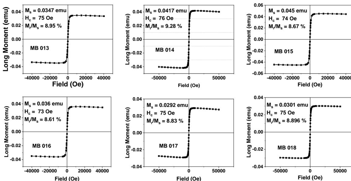
**Figure 8.** Hysteresis loops measured at 300 K for samples MB013-MB017.
