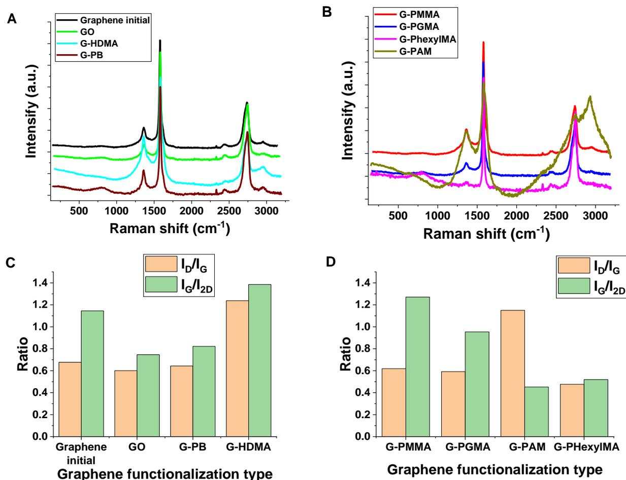
**Figure 5.** RAMAN spectra,  $I_D/I_G$ , and  $I_G/I_{2D}$  ratio for the functionalized graphene: initial graphene and functional groups modified graphene (A,C), polymer functionalized graphene (B,D).
