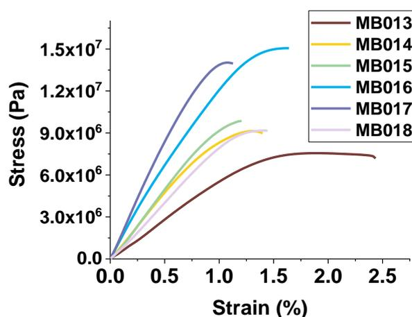
Figure 10. Comparative stress-strain plots of the thin films.
