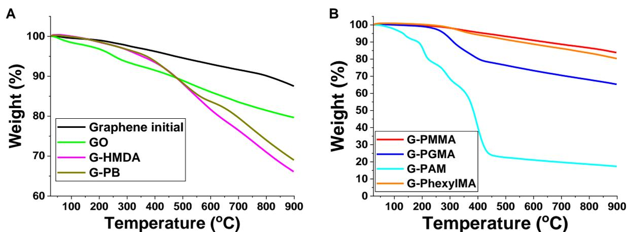
**Figure 4.** TGA analyses of the functionalized graphene (A) small molecules/functional groups and (B) polymers.
