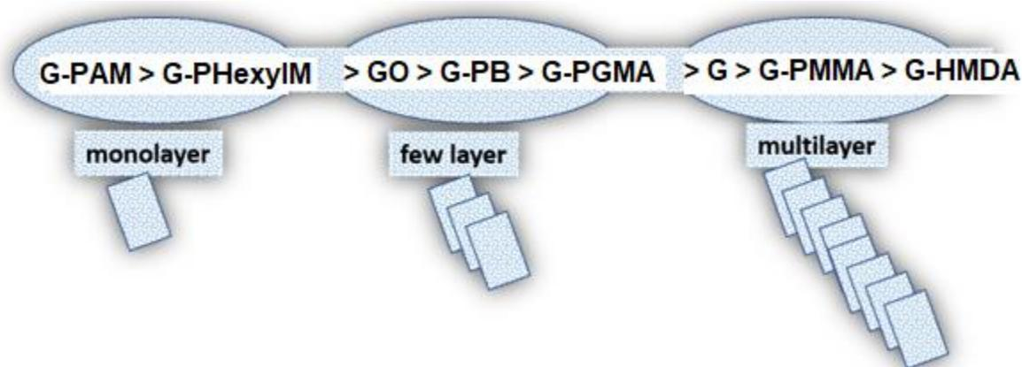
**Scheme 1.** Graphical representation of the graphene stacks' thickness depending on the functionalization technique.
