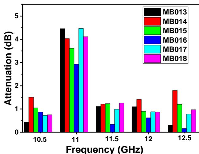
Figure 6. Electromagnetic shielding attenuation dependence on the frequency.
