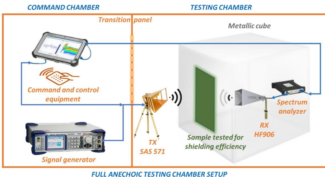
**Figure 1.** Experimental setup for assessing shielding efficiency of the samples.
