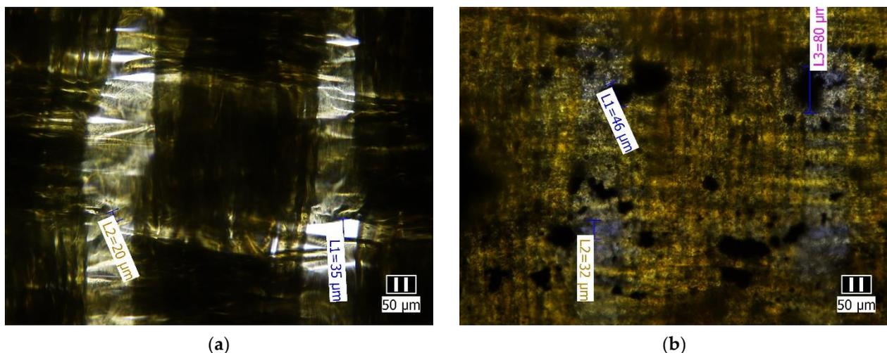
**Figure 2.** Optical microscopy images: (a) unmodified textile material; (b) GO-modified epoxy resin.
