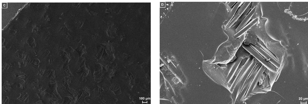
**Figure 3.** SEM images of unmodified textile material (A,B) and GO epoxy resin-coated textile material (C,D).
