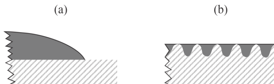
Figure 3. Illustration of the water droplet on a smooth hydrophilic surface (a) and superhydrophilic surface of rich morphology on the sub-micrometer scale (b).
