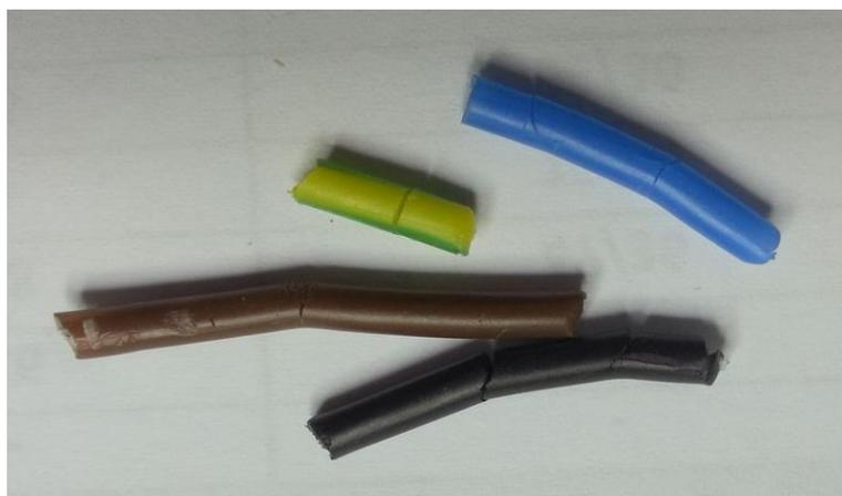
**Figure 5.** Appearance of cracks in XLPE insulations (IC1 cable) after three years of irradiation in SPS.
