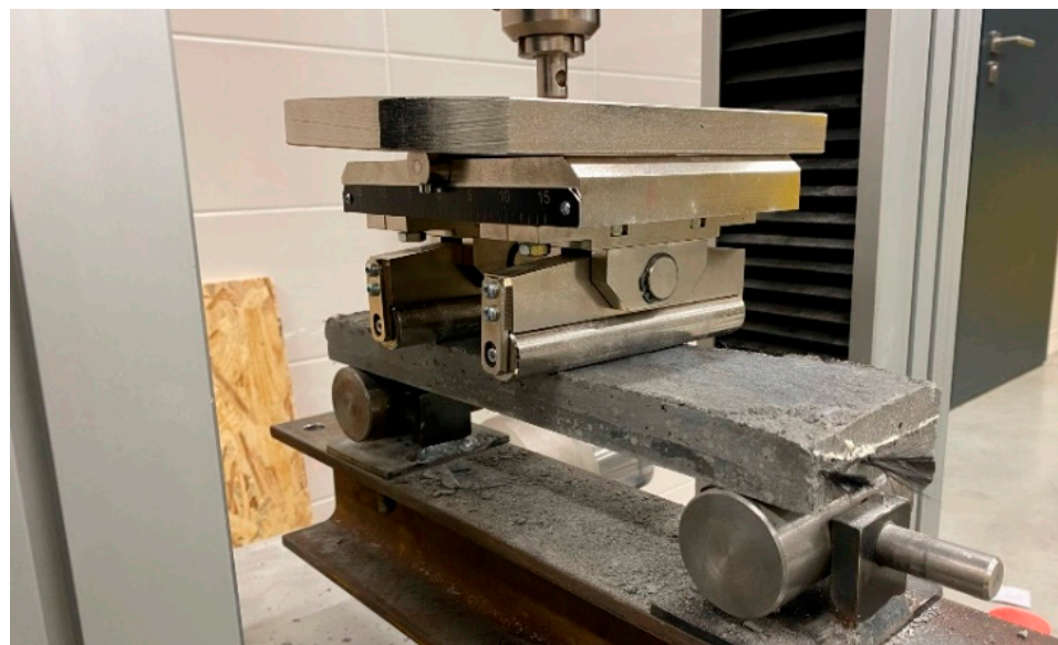
Figure 5. Test specimen place in the mechanical press for four-point bending test.
