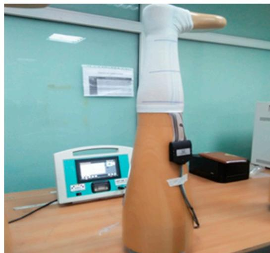
**Figure 4.** A medical stocking tester (MST) and MK V pressure measurement device.
