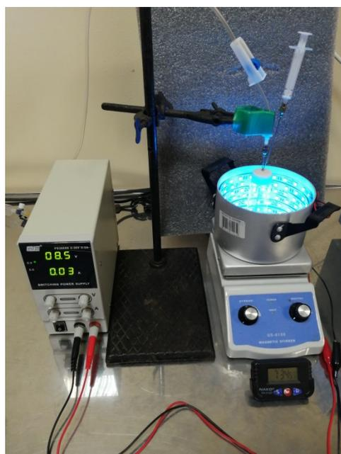
**Figure 2.** Experimental set-up for the photoiniferter polymerization.
