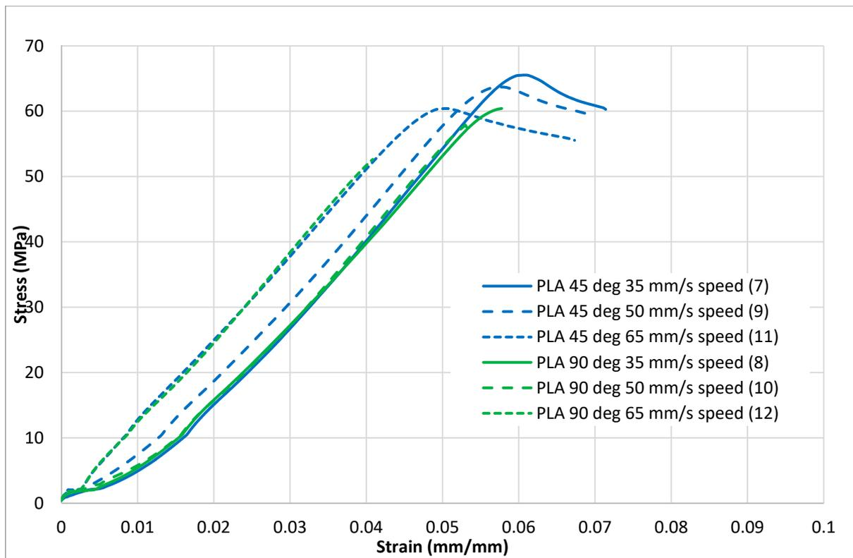
Figure 4. Tensile test results (stress–strain curves) for the standard PLA material.
