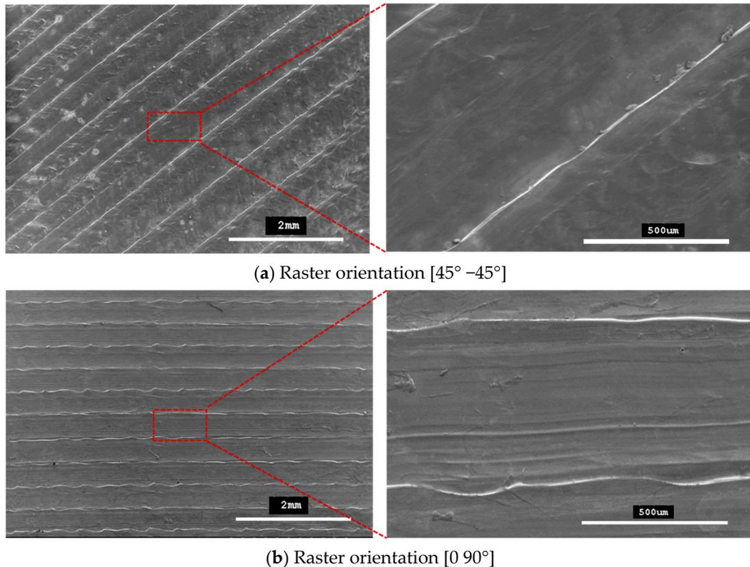
**Figure 9.** SEM micrographs showing printing patterns on specimens fabricated with (a) raster orientations ( $45^\circ - 45^\circ$ ) and (b) raster orientations ( $0^\circ - 90^\circ$ ).
