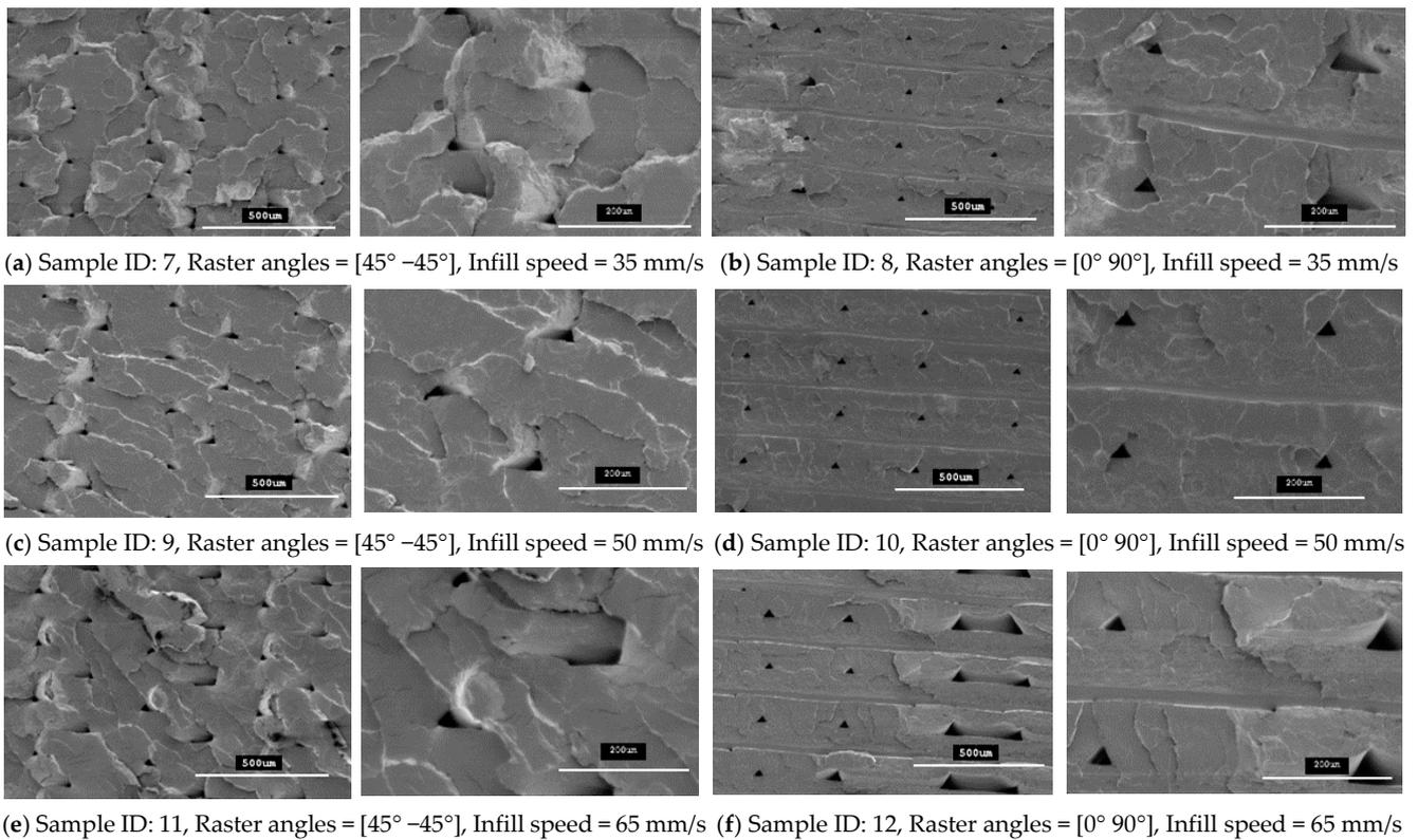
**Figure 10.** SEM images of the fractured interface of tensile specimens fabricated with two different raster orientations ( $45^\circ -45^\circ$  and  $0^\circ 90^\circ$ ) with three infill speeds for the PLA material type.
