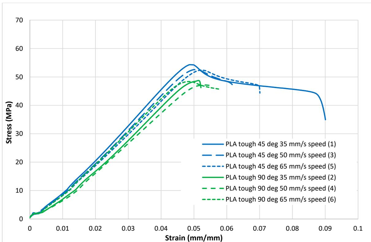
Figure 5. Tensile test results (stress–strain curves) for the tough PLA material.
