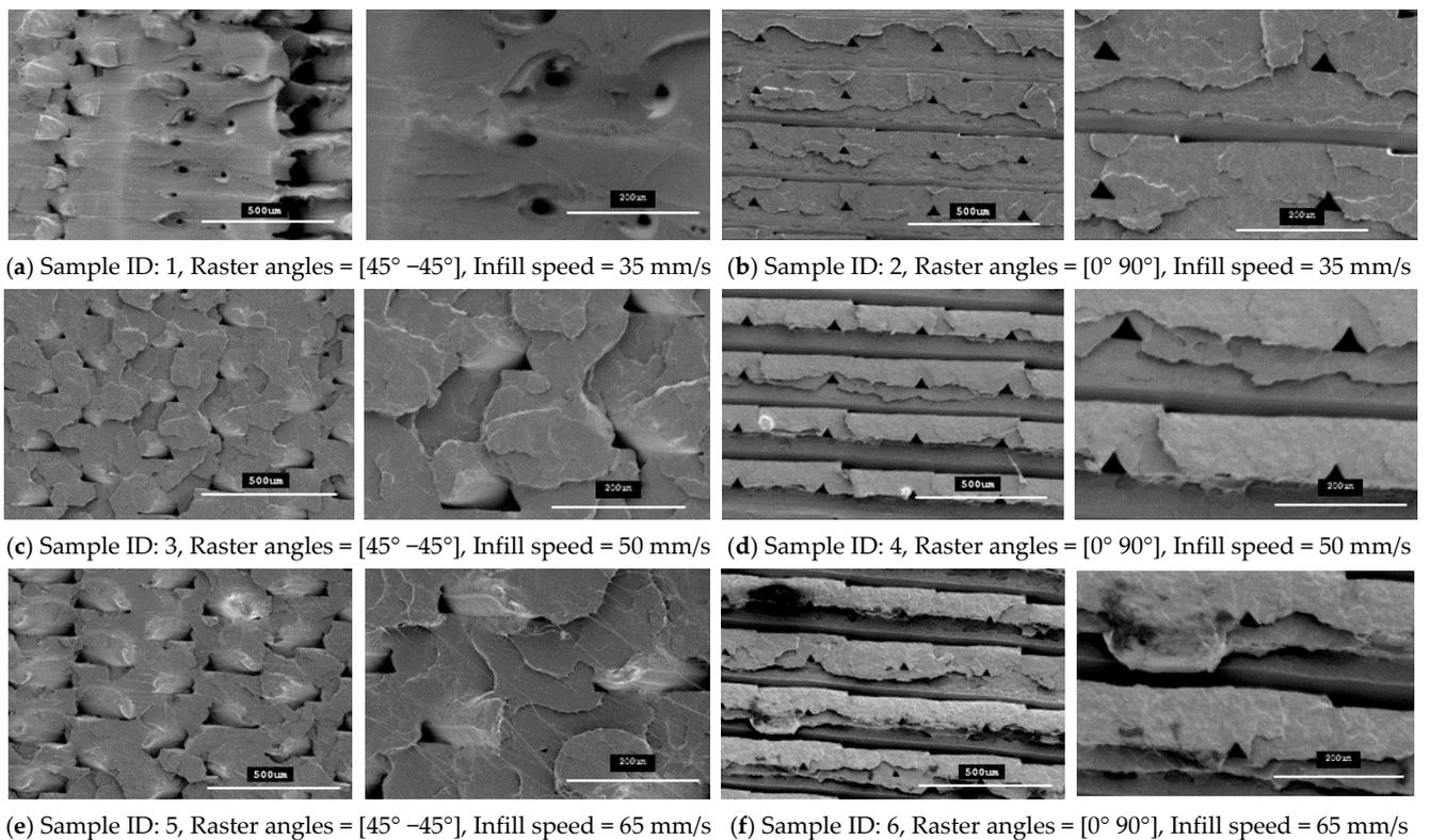
**Figure 11.** SEM images of the fractured interface of tensile specimens fabricated with two different raster orientations ( $45^\circ -45^\circ$  and  $0^\circ 90^\circ$ ) with three infill speeds for the tough PLA material type.
