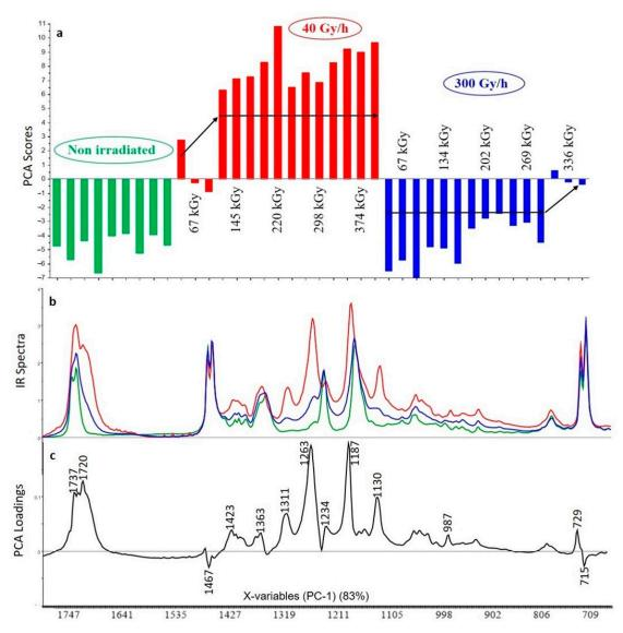
**Figure 6.** PCA scores (**a**), FTIR spectra for highest dose (**b**) and PCA loadings (**c**) of the first principal component (PC1) for the analysis of XLPE with Irganox PS802 (green: unaged samples, red: samples irradiated at 40 Gy/h, blue: samples irradiated at 300 Gy/h).
