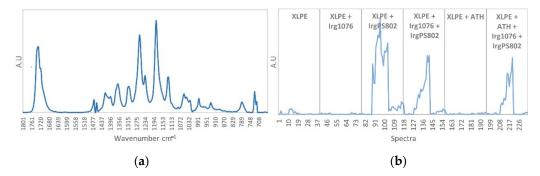
**Figure 13.** (a) IrgPS802 degradation products pure spectrum. (b) IrgPS802 degradation products concentration profile.
