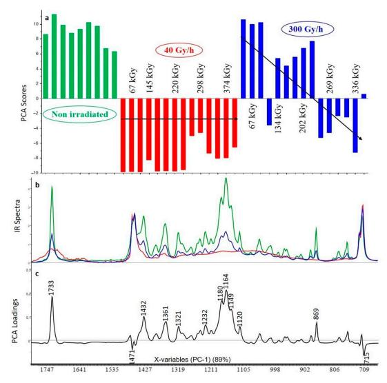
**Figure 5.** PCA scores (**a**), FTIR spectra for highest dose (**b**) and PCA loadings (**c**) of the first principal component (PC1) for the analysis of XLPE with Irganox 1076 (green: unaged samples, red: samples irradiated at 40 Gy/h, blue: samples irradiated at 300 Gy/h).
