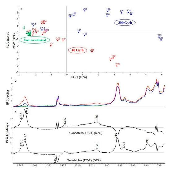
**Figure 9.** PCA scores (**a**), FTIR spectra for highest dose (**b**) and PCA loadings (**c**) of the first and second principal components (PC1 and PC2) for the analysis of XLPE with ATH (green: unaged samples, red: samples irradiated at 40 Gy/h, blue: samples irradiated at 300 Gy/h).
