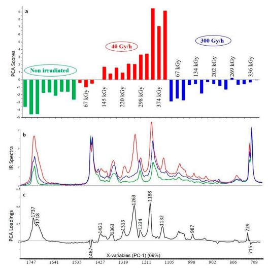
**Figure 8.** PCA scores (**a**), FTIR spectra for highest dose (**b**) and PCA loadings (**c**) of the first principal component (PC1) for the analysis of XLPE with Irganox 1076 and Irganox PS802 (green: unaged samples, red: samples irradiated at 40 Gy/h, blue: samples irradiated at 300 Gy/h).
