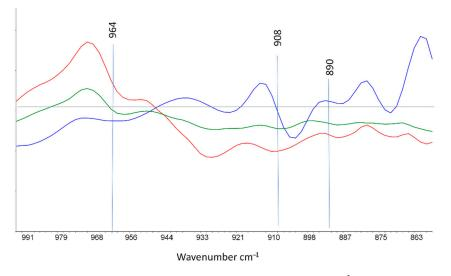
**Figure 4.** First derivative FTIR spectra in the range 995–860 cm<sup>-1</sup> of XLPE irradiated at 374 kGy and 40 Gy/h (red), XLPE irradiated at 336 kGy and 300 Gy/h (green), and non-irradiated XLPE (blue).
