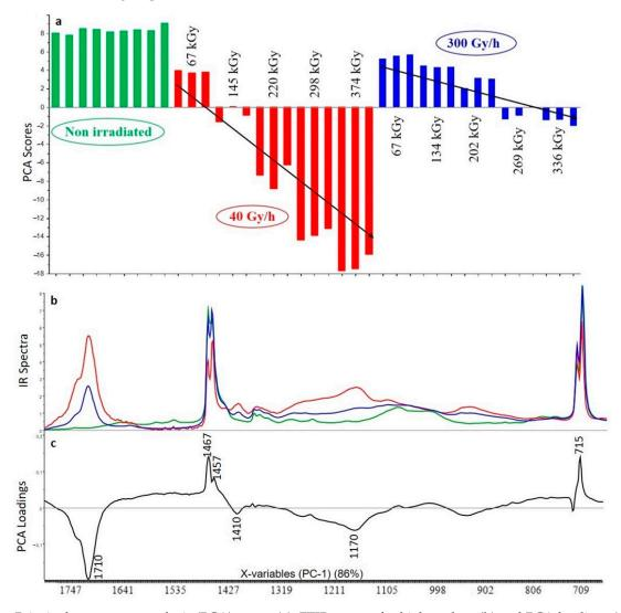
**Figure 3.** Principal component analysis (PCA) scores (**a**), FTIR spectra for highest dose (**b**) and PCA loadings (**c**) of the first principal component (PC1) for the analysis of XLPE polymer without additive (green: unaged samples, red: samples irradiated at 40 Gy/h, blue: samples irradiated at 300 Gy/h).
