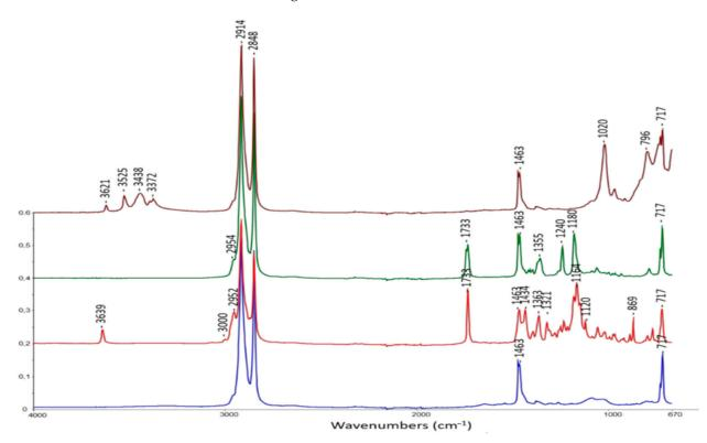
**Figure 2.** Attenuated total reflectance-Fourier transform infrared (ATR-FTIR) spectra of unaged materials: crosslinked polyethylene (XLPE, blue), XLPE + Irganox 1076 (red), XLPE + Irganox PS802 (green) and XLPE + alumina trihydrate (ATH, brown).
