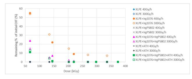
**Figure 17.** Remaining percentages of initial oxidative induction time (OIT) for the different samples (full markers: samples irradiated at 40 Gy/h, empty markers: samples irradiated at 300 Gy/h).
