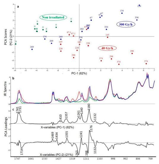
**Figure 10.** PCA scores (**a**), FTIR spectra for highest dose (**b**) and PCA loadings (**c**) of the first and second principal components (PC1 and PC2) for the analysis of XLPE with ATH, Irganox 1076 and Irganox PS802 (green: unaged samples, red: samples irradiated at 40 Gy/h, blue: samples irradiated at 300 Gy/h).
