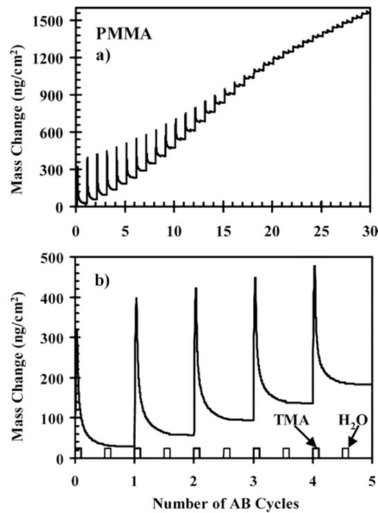
**Figure 5.** Mass change measurements by QCM versus number cycles of Al<sub>2</sub>O<sub>3</sub> ALD on PMMA at 85 °C for (a) 30 and (b) 5 cycles (reprinted with permission from [40], Copyright (2005) American Chemical Society).
