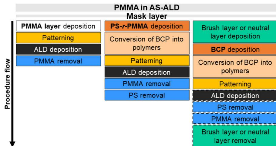
**Figure 21.** PMMA in an AS-ALD process, where the block copolymers are polystyrene-*random*-poly(methylmethacrylate) (PS-*r*-PMMA) or polystyrene-*block*-poly(methylmethacrylate) (PS-*b*-PMMA).
