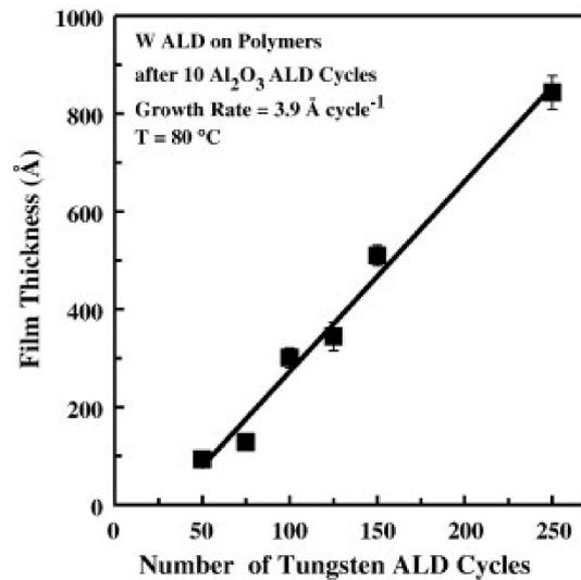
**Figure 13.** Profilometry measurements of W ALD film thickness on different polymers vs. the number of W ALD cycles.  $\text{Al}_2\text{O}_3$  ALD was used as a seed layer (10 ALD cycles) (reprinted from [64], Copyright (2008), with permission from Elsevier).
