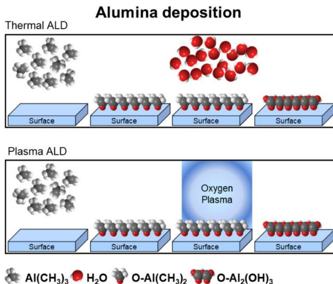
**Figure 17.** Schematic representation of one cycle of  $\text{Al}_2\text{O}_3$  by thermal ALD and plasma ALD techniques. In plasma ALD, the  $\text{H}_2\text{O}$  co-reactant is replaced with a plasma exposure (e.g.,  $\text{O}_2$  plasma) to grow metal oxides.
