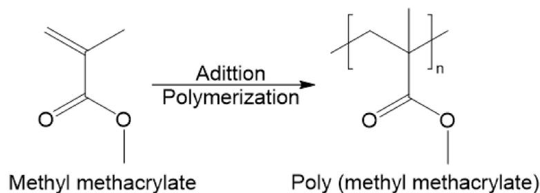
**Figure 3.** Synthesis of PMMA by addition polymerization of MMA (adapted from [1]).
