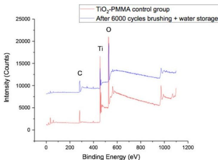
**Figure 12.** XPS results of coated PMMA unbrushed (red) and brushed (blue), storage in water and brushed again after 5 months [48]. PMMA has great mechanical properties and low toxicity for the dental prosthesis fabrication (this work by Ghaith Darwish is licensed under a Creative Commons Attribution (CC BY 4.0)).
