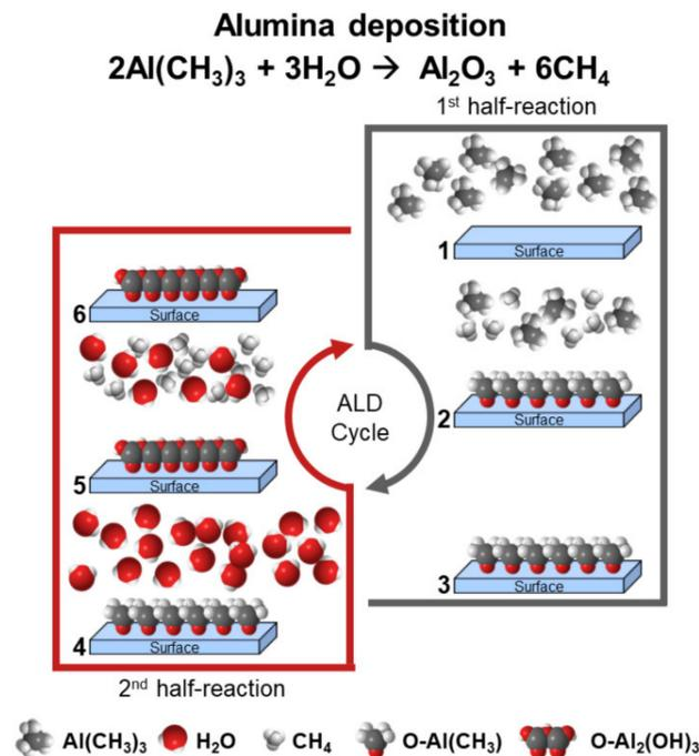
**Figure 2.** Schematic representation of the ALD formation of the first  $\text{Al}_2\text{O}_3$  monolayer from: (1) TMA pulsing; (2) TMA chemisorption in the surface (first half-reaction); (3) after purging of unreacted TMA and methane; (4) water pulsing; (5) water chemisorption on the by-product from the first half-reaction; and (6) after purging of unreacted water and methane.
