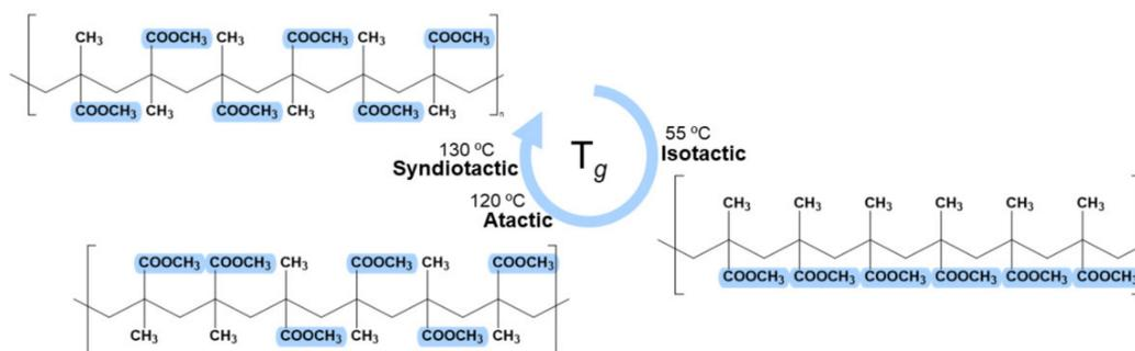
**Figure 4.** PMMA tacticities: isotactic, syndiotactic, and atactic and respective glass transition temperature. The tacticities values were collected from [44].
