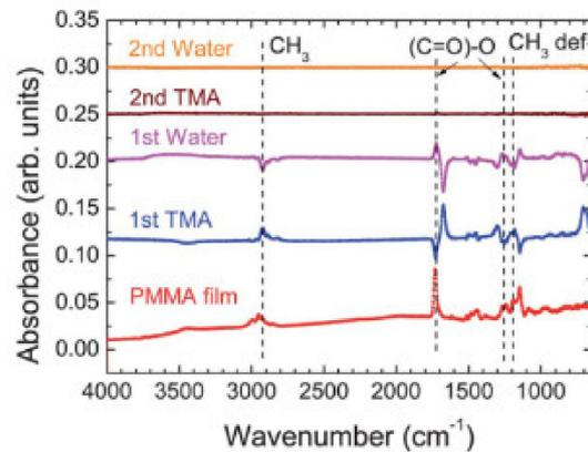
**Figure 6.** In-situ FTIR analysis of uncoated PMMA spin-coated onto Si, first, and second ALD half-reactions. Al<sub>2</sub>O<sub>3</sub> coating was made from TMA and H<sub>2</sub>O at 80 °C. A FTIR run followed each half-cycle, and between half-cycles, the reactor was purged for 10 s (republished with permission of Be Gong, from [52]; permission conveyed through Copyright Clearance Center, Inc.).
