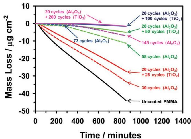
**Figure 14.** Mass loss of uncoated and coated PMMA with  $\text{Al}_2\text{O}_3$  and  $\text{Al}_2\text{O}_3/\text{TiO}_2$  when exposed to vacuum UV radiation over time (reprinted with permission from [65], Copyright (2010) American Chemical Society).
