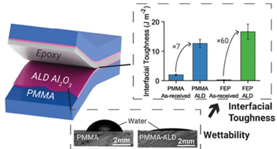
**Figure 8.** Thermoplastic-epoxy resin with the double Al<sub>2</sub>O<sub>3</sub> coating; wettability test of a water droplet in coated and uncoated PMMA surface, and the interfacial toughness of PMMA and fluorinated ethylene propylene (FEP) (wedge test) (reprinted with permission from [54], Copyright (2019), American Chemical Society).
