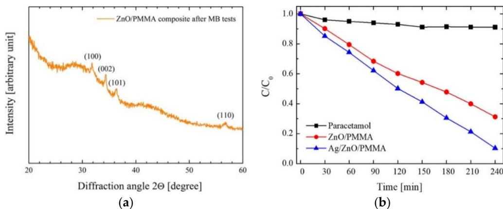
**Figure 11.** XRD pattern of ZnO/PMMA composite after the seven MB discoloration runs [62]. (a) Degradation of paracetamol drug as a function of irradiation time for paracetamol alone (squares), paracetamol with ZnO/PMMA (circles), and paracetamol with Ag/ZnO/PMMA (triangles) samples (b), under UV illumination [61] (both works by Alessandro Di Mauro are licensed under a Creative Commons Attribution (CC BY 4.0)).
