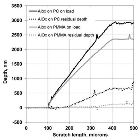
**Figure 7.** On-load and residual depth curves for  $\text{Al}_2\text{O}_3/\text{PMMA}$  and  $\text{Al}_2\text{O}_3/\text{PC}$  (polycarbonate) after the nanoscratch. The test was repeated five times per sample; each scratch had 500  $\mu\text{m}$  of length, at a scanning velocity of 10  $\mu\text{m}/\text{s}$ , and a ramped load varying from 0.1 mn to 60 mn (reprinted with permission from [53], Copyright 2012, American Vacuum Society).
