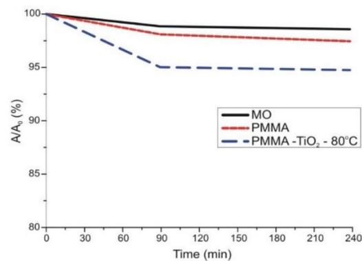
**Figure 10.** Photocatalytic efficiency of the amorphous TiO<sub>2</sub>. After 90 min, the methylene orange dye degraded 5% under UV-A illumination [adapted from [59], this work by Orsolya Kéri is licensed under a Creative Commons Attribution (CC BY 4.0)].
