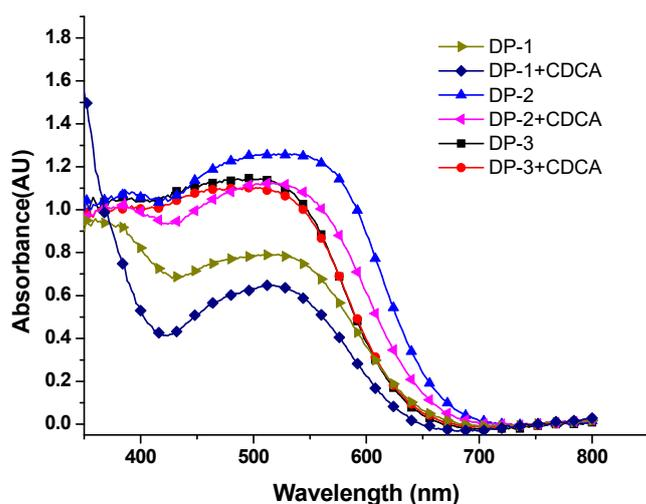
**Figure 3.** The absorption spectra of DP-1, DP-2, and DP-3 on TiO<sub>2</sub> films.
