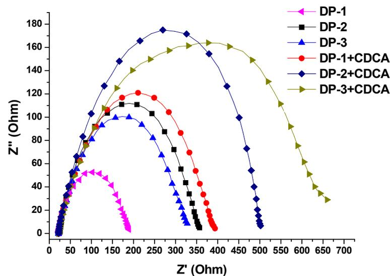
**Figure 7.** Nyquist plots of DSSCs based on dyes measured at  $-0.7$  V forward bias in the dark.
