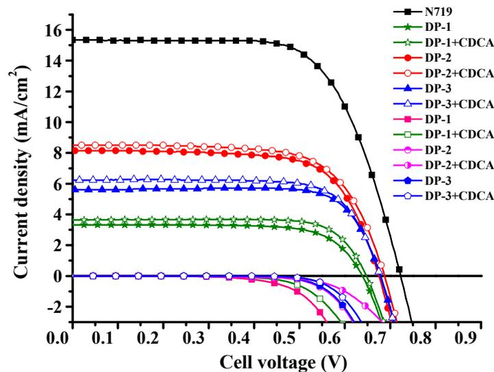
Figure 5. *J*–*V* curves and dark currents of dye-sensitized solar cells (DSSCs) based on the dyes.
