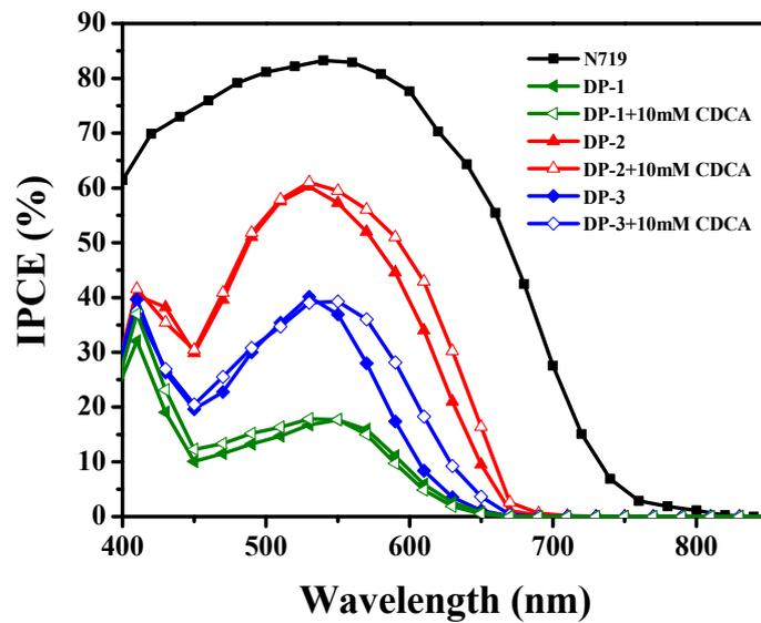
**Figure 6.** Incident monochromatic photo-to-current conversion efficiency (IPCE) plots of the DSSCs using the dyes and N719.
