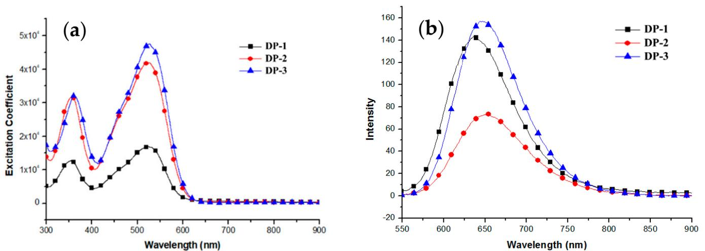
Figure 2. (a) Absorption spectra of dyes in THF solutions; (b) the emission spectra of the dyes in THF.
