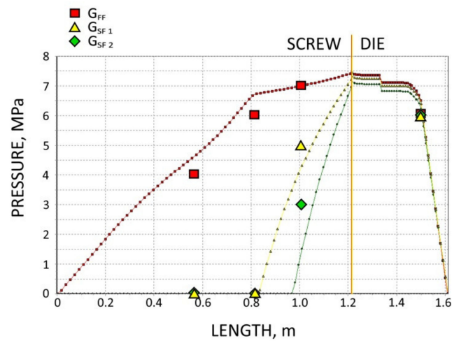
Figure 13. Validation of pressure computation: WPC of WF/PP = 20/80, n = 70 rpm.
