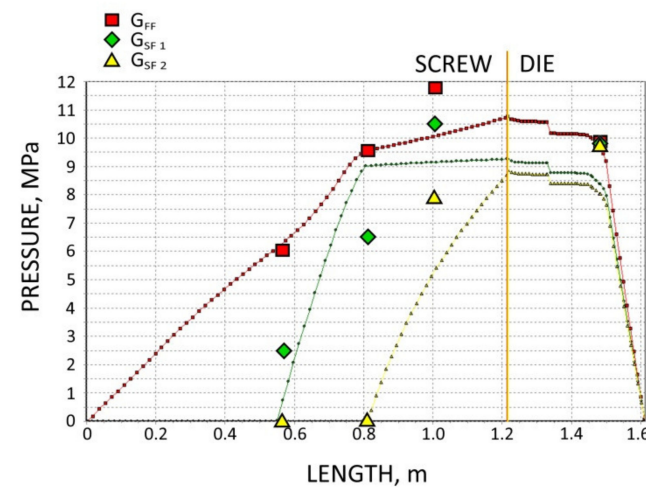
Figure 15. Validation of pressure computation: WPC of WF/PP = 40/60, n = 70 rpm.
