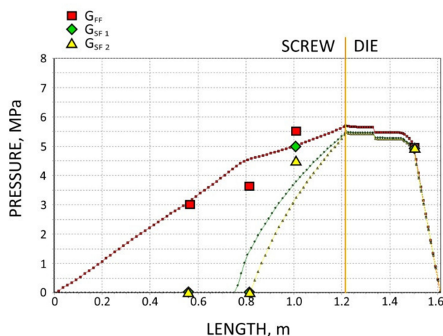
Figure 12. Validation of pressure computation: WPC of WF/PP = 20/80, n = 30 rpm.
