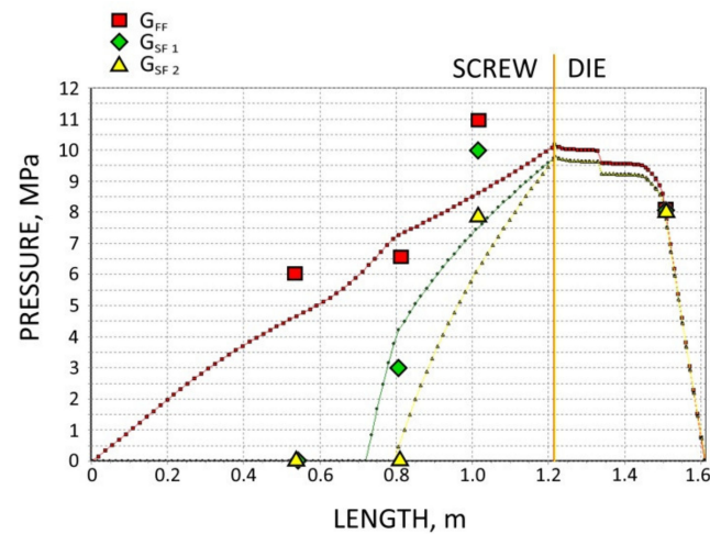
Figure 14. Validation of pressure computation: WPC of WF/PP = 40/60, n = 30 rpm.
