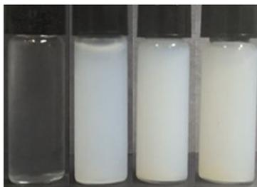
**Fig. S1.** Photographs of the typical hydrogels at 52 °C. From left to right: hydrogels of PAAc-co-PAAm, PAAc/PAAm/CNC<sub>1</sub>, PAAc/PAAm/CNC<sub>2</sub>, and PAAc/PAAm/CNC<sub>3</sub>.
