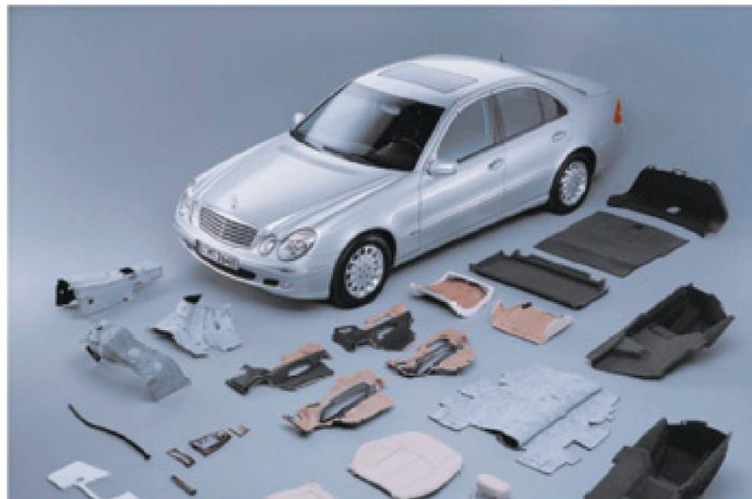
**Figure 4.** Automobile components fabricated with natural fiber related composites. Reprinted with permission from the publisher [16]. Open access.
